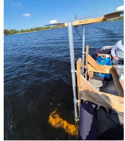
(b) Receiver array mounted over the side of a boat
