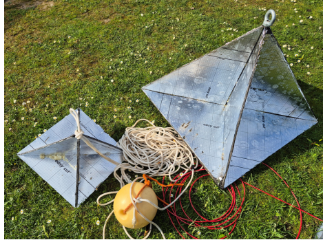
Figure 4.19: Image of two corner reflectors to be imaged. The radii of the corner reflectors are 20 cm and 40 cm, respectively, with estimated target strengths of -24 dB and -12 dB.
