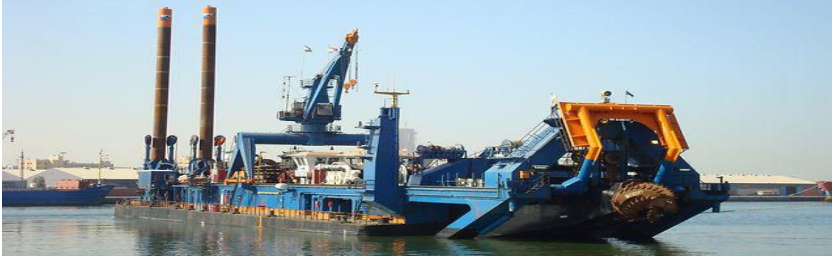
FIGURE 28: CUTTER SUCTION DREDGER “CASTOR (VAN OORD)”
