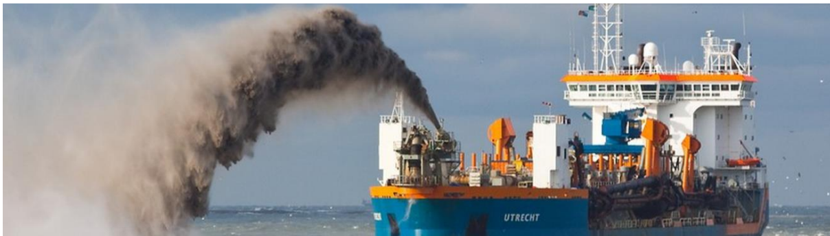
FIGURE 82: TRAILING SUCTION HOPPER DREDGER "UTRECHT".
