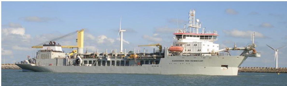
FIGURE 27: TRAILING SUCTION HOPPER DREDGER “ALEXANDER VON HUMBOLDT (JAN DE NUL)”.
