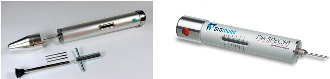
figure 3-13: two types of penetrometers, left: Pylodyn (Istemi, n.d.), right: Specht (Profound, 2017)
