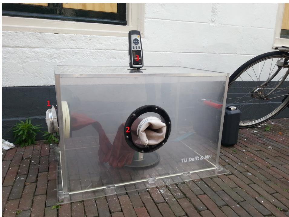
Figure A.2: The acrylic box made and used by the TU Delft bachelor group Hockers et al. (2013) [1] and van Doeveren et al. (2014) [2], shown here without the internal mechanism. Picture by van Doeveren et al. (2014) [2]
