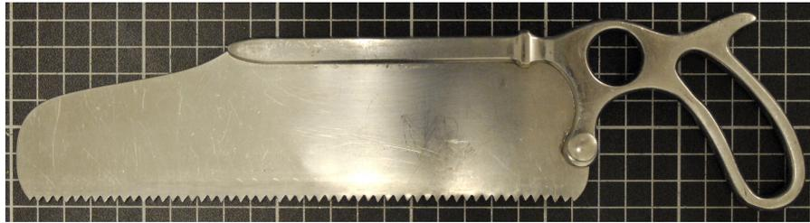
Figure A.7: Satterlee type bone saw used in Exp. 6 'DCB' and Exp. 7 'GCB', with a 200x60x0.8mm, 9 teeth per inch saw blade (FH325R, Aesculap AG, Germany). Each square of the gridline background is 10x10mm.
