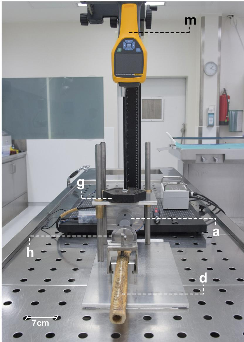
Figure A.6: Front view of the setup; the sliding platform was placed directly on a 100x310cm custom built autopsy table that was equipped with a built-in ventilation system with a ventilation capacity of 3000 m<sup>3</sup>/h through 252, 2cm diameter holes spaced 7cm apart.
