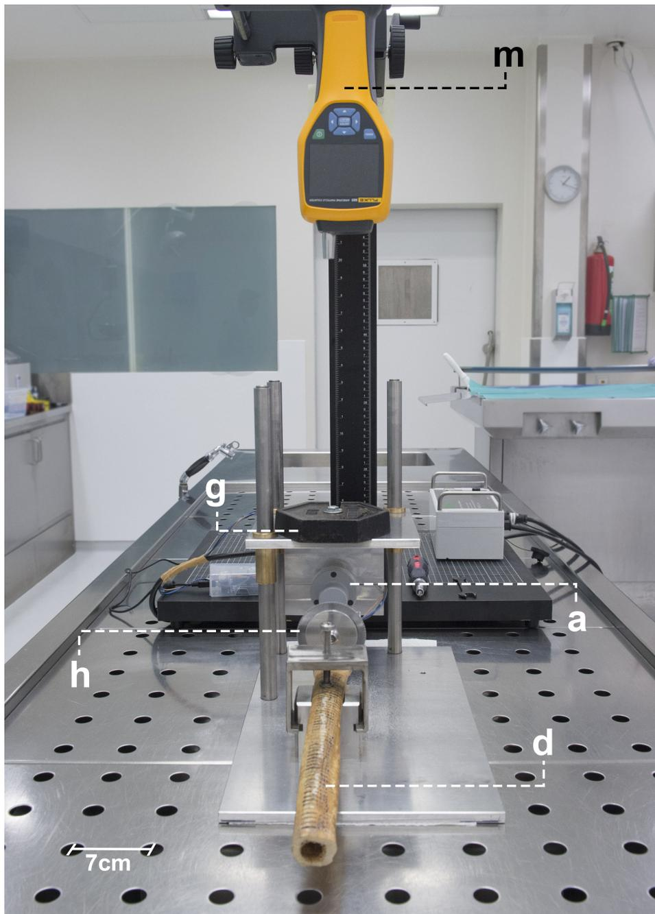
Figure 3.6: Front view of the setup; the electric oscillating saw (a) mounted under the weighted (g) sliding platform, with the saw blade (h) ready to make a test cut in the bone (d). The whole setup was placed directly on a 100x310cm custom built autopsy table that was equipped with a built-in ventilation system with a ventilation capacity of 3000 m<sup>3</sup>/h through 252, 2cm diameter holes spaced 7cm apart.
