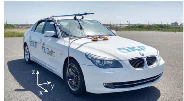
Fig. 9. Instrumented test vehicle including load sign convention.
