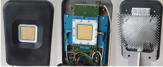
FIGURE 3. The active mm-wave (26 GHz) dual-linear polarized phased array prototyped by NXP and TNO [32], [33].
