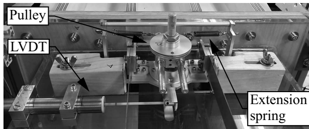
(a) Pitch mechanism
