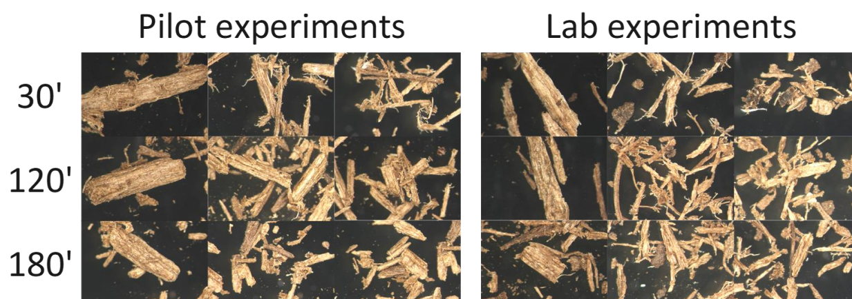
Figure 3.S3. Visual analysis at the microscope of the surface of the LHW pretreated material at different pretreatment times at lab and pilot scales.
