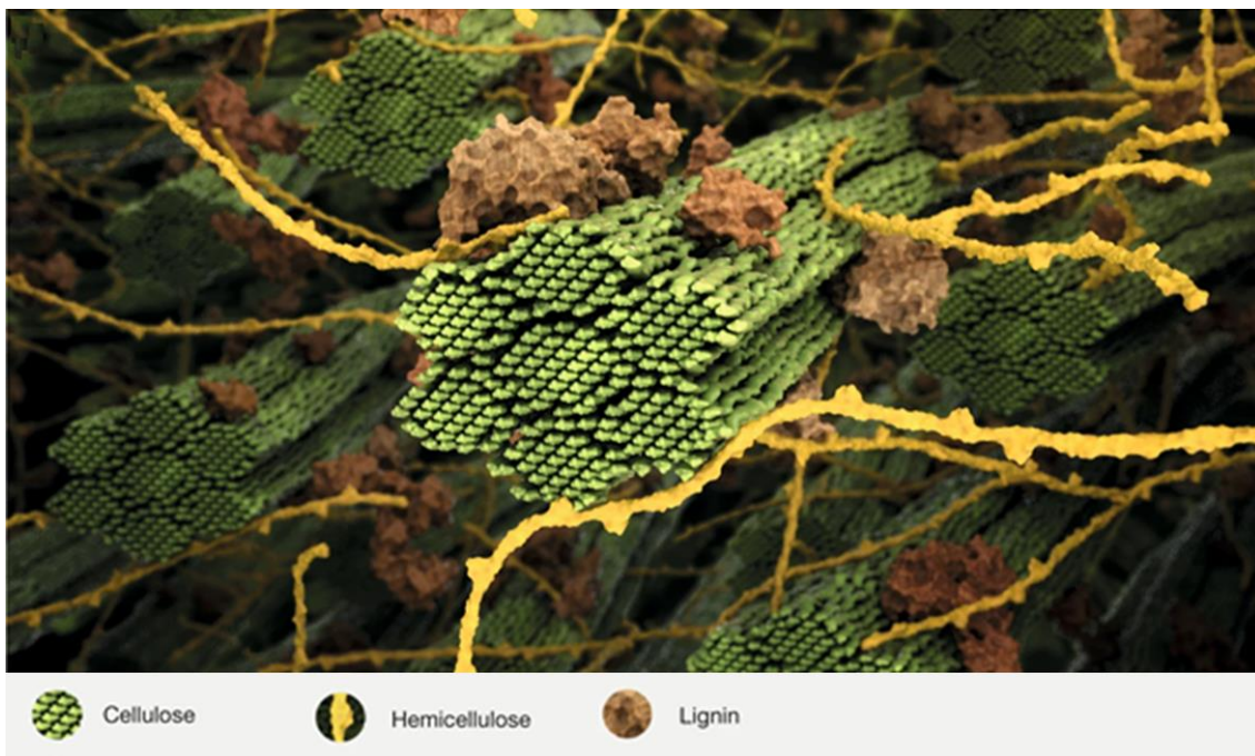
Figure 1.2. Representation of lignocellulosic biomass structure, including cellulose (green, with seven micro-fibrils depicted as forming a fibre), hemicellulose (yellow) and lignin (brown) (Adapted with permission from Petridis and Smith (2018)).
