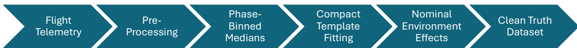
Figure 6.1: Nominal thermal truth generation workflow used to produce the clean multichannel reference for later anomaly injection.
