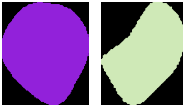
Figure 4. Two examples of strawberry segments. Left: strawberry segment with a circularity of 0.263: not occluded; right: strawberry segment with a lower circularity of 0.245: occluded.
