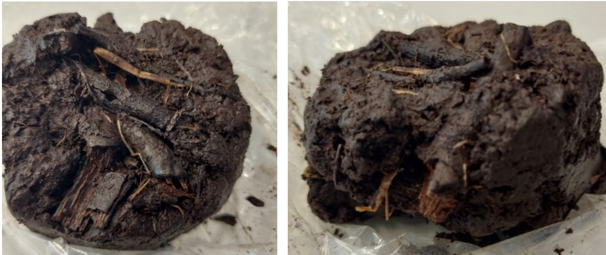
Figure A2.1: Left: top view of peat sample clearly shows undecomposed wood and fibres.
