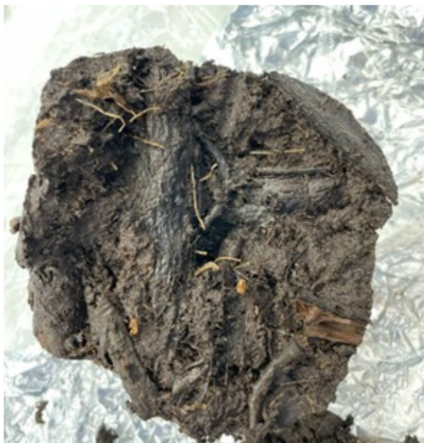
Figure A2.11: Cross-section of peat cylinder reveals the observations made in the CT scan where wooden branches are clearly visible.
