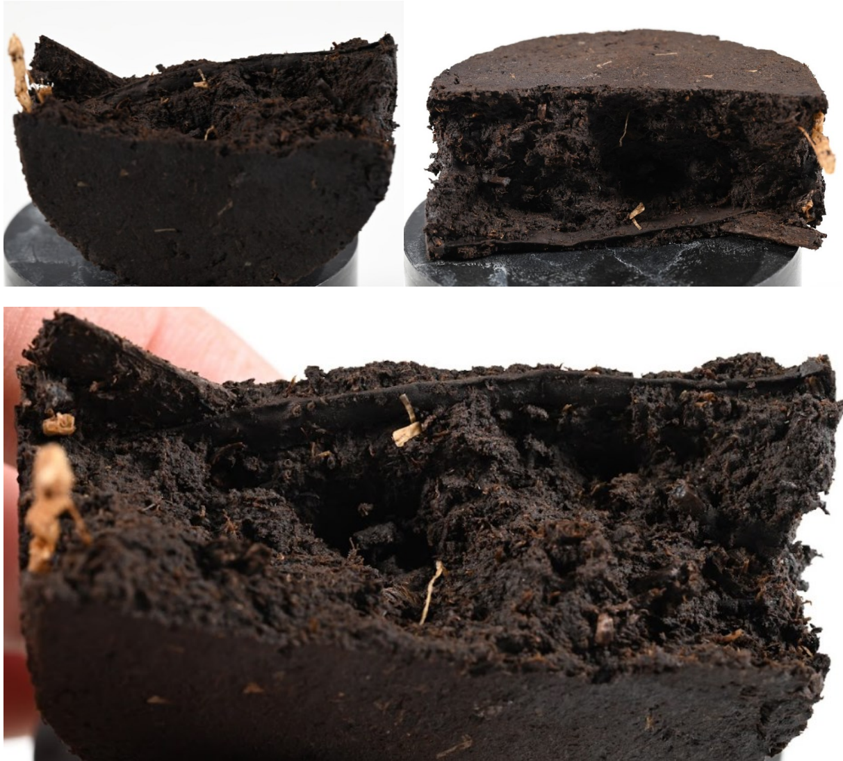
Figure A12. 3: After stopping the CRS test and dismantling the soil sample the presence of wood was confirmed. Note that wood much larger than the peat fibres is clearly visible in the soil sample.
