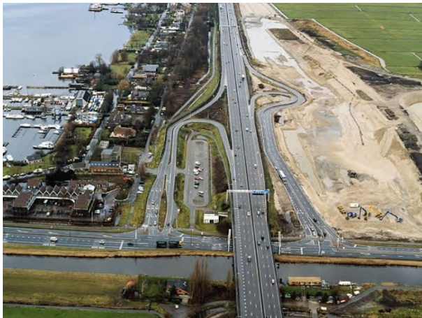
Figure 3.8: Widening of the A2. The embankment construction connecting Vinkeveen to the A2 is under construction on the right side of the image [Rijkswaterstaat].
