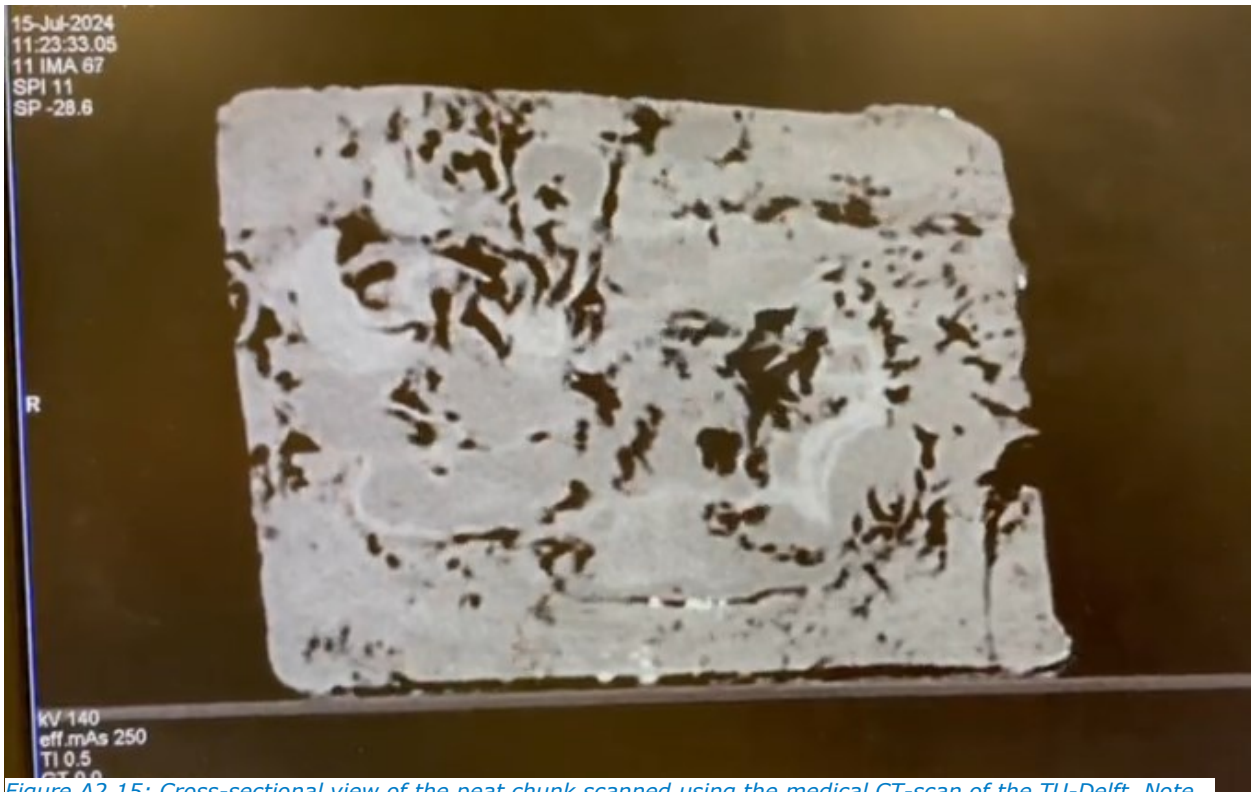
Figure A2.15: Cross-sectional view of the peat chunk scanned using the medical CT-scan of the TU-Delft. Note the large areas in black indicating pore volumes. This underlines the calculated void ratio of the Zegveld peat.
