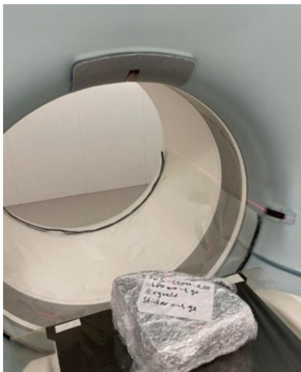
Figure A2.13: The medical CT-scan allows large part of the peat layer to be scanned.
