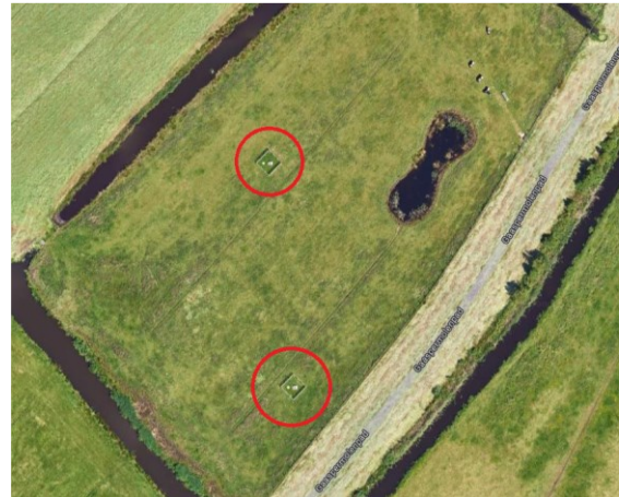
Figure 3.19: Satellite view of the peat meadow near Gaasp with the locations of the corner reflectors marked in red.
