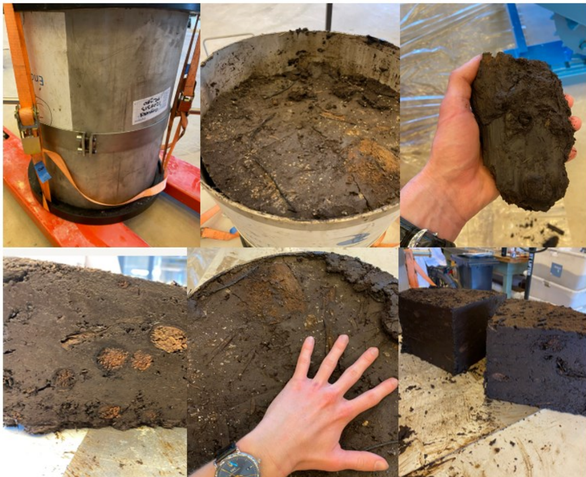
Figure A1.1: Extraction process of Zegveld peat used in CRS testing.
