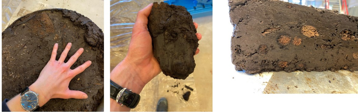
Figure 4.2: Wood can clearly be identified in the Zegveld peat used for CRS testing.
