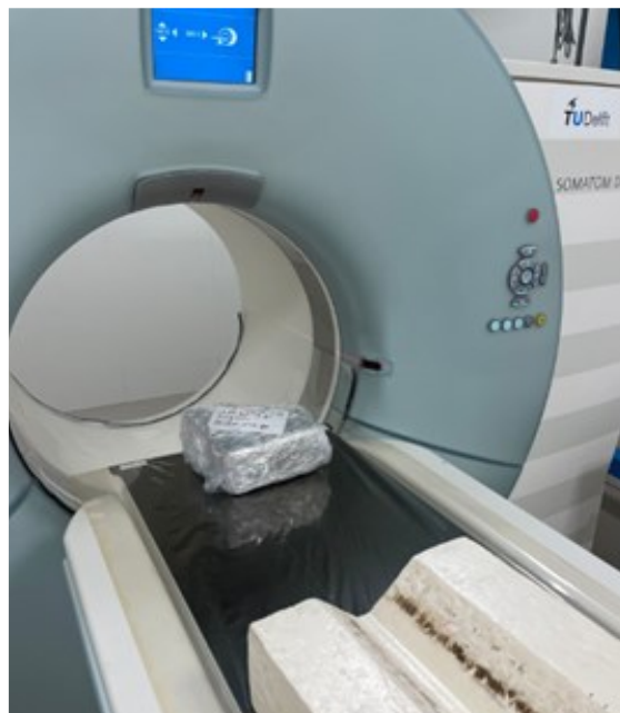
Figure A2.12: Medical CT-scan of peat cylinder at the laboratory of the TU-Delft.
