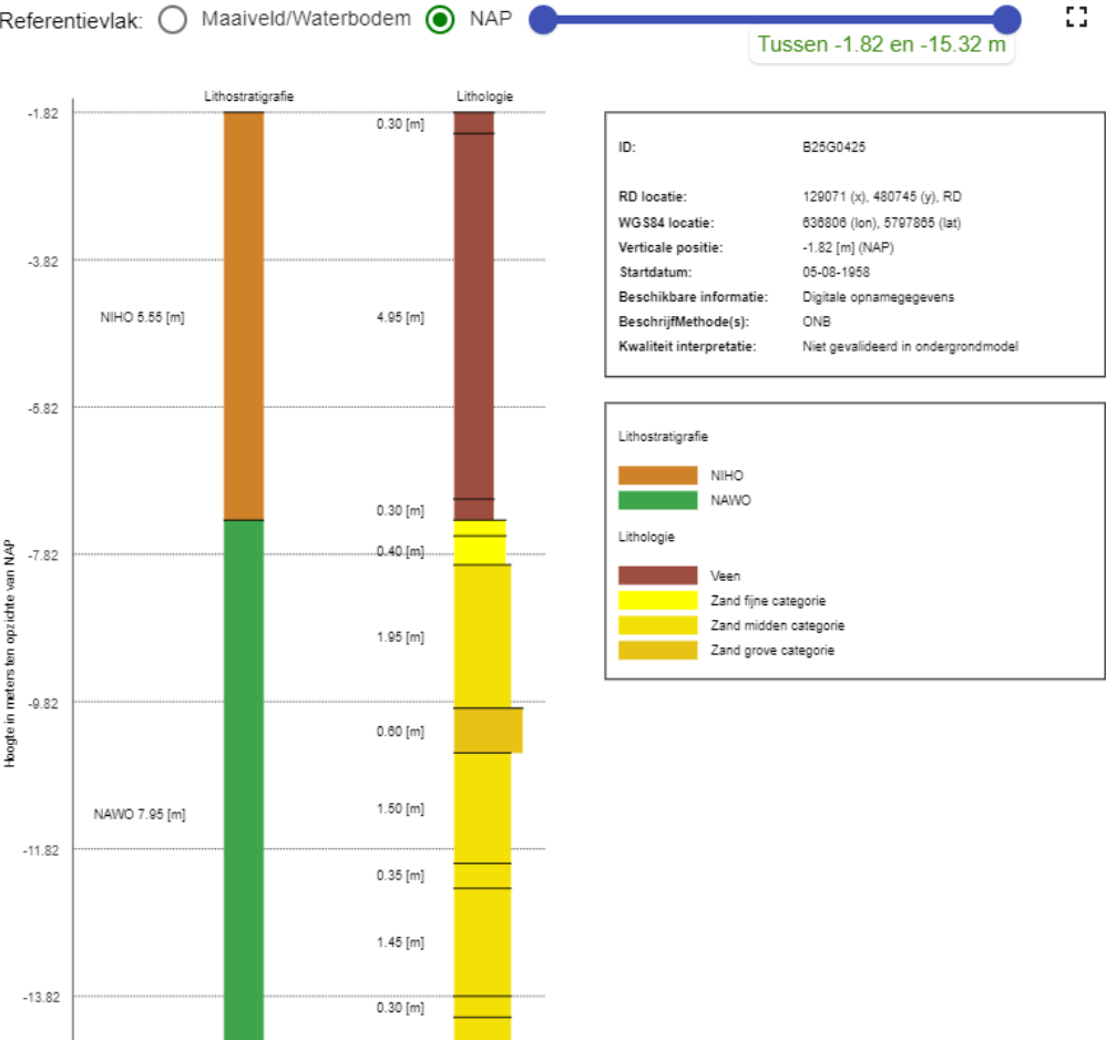
Figure A18.1: Bore profile next to the embankment connecting Vinkeveen to the A2. Measurement depths are with respect to Nap. Observe the 6 meter thick peat later directly below surface level.
