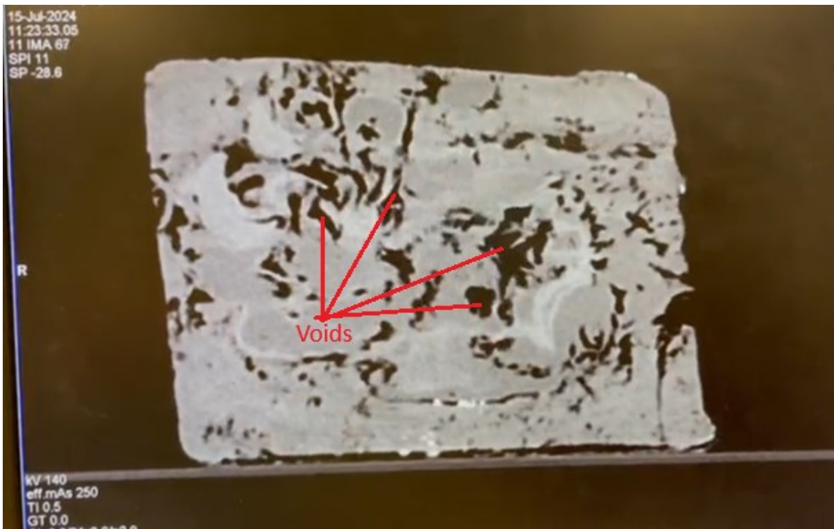
Figure A2.16: Cross-sectional view of the peat chunk scanned using the medical CT-scan of the TU-Delft with annotated voids.
