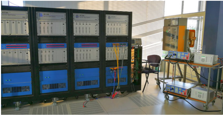
Fig. 3.3 RTDS with SMT components
