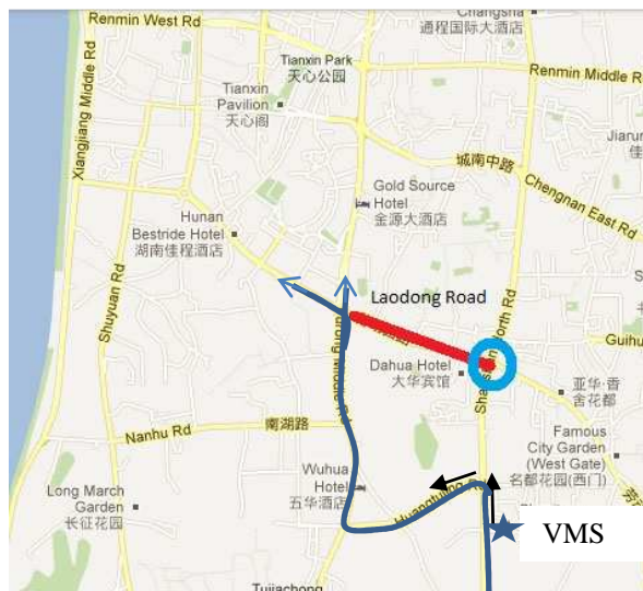
23 FIGURE 6 Map of the application area with the queue spillback (red line) on the Laodong road. The 24 critical intersection is shown with a blue circle. The best rerouting is to turn left already to the 25 Huangtuling Road
