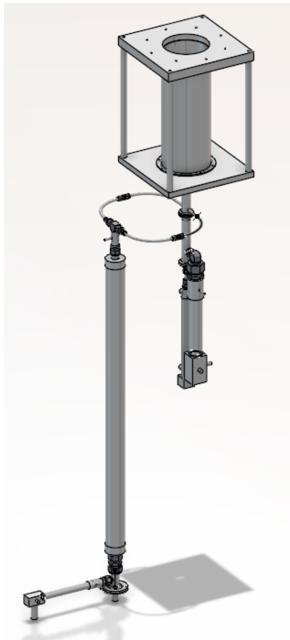
Figure A.1: Complete System of Proposed Swirl Burner. The long tube on the left is the fuel-prevaporizer system with heater installed horizontally. The AAI line pass through the heater installed vertically on the center, towards the swirler plenum. The main air line is on the right with the vertical heater and injected through an elbow to the swirler plenum.
