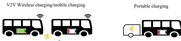
**FIGURE 18.** E-bus alternative charging system.
