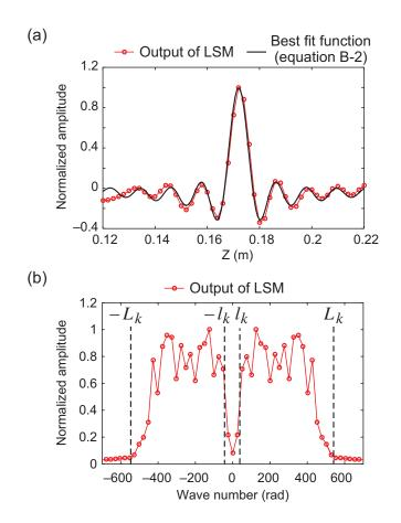
Figure B-1: (a) An example of the estimation of  $L_k$  and  $l_k$  in equation B-2. The red line shows the output of LSM at x = 0.15 m followed by normalization of the amplitude, and the black line shows the best-fit curve using equation B-2 with  $(L_k, l_k) = (543.50, 40.84)$ .
