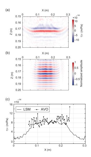
Figure 8: (a) Imaging results on laboratory experimental data of a homogeneously wet fracture using the proposed LSM (50–500 KHz). (b) Imaging result using initial gradient. (c) Estimated normal fracture compliance along the fracture from the proposed LSM and the AVO inversion from Minato et al. (2018).
