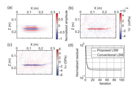
Figure 2: Imaging results for SH wavefield; (a) Initial gradient without inversion, (b) proposed LSM involving linear-slip theory, and (c) conventional LSM without linear-slip theory.
