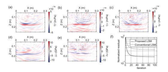
Figure 3: Imaging results for P-SV wavefield using the proposed LSM; (a) tangential compliance, (b) normal compliance, and (c) coupling compliance. (d)–(e) Imaging results using the conventional LSM for the perturbation in  $\lambda$  and  $\mu$ . (f) Residuals at each CG iteration using the proposed LSM and the conventional LSM.
