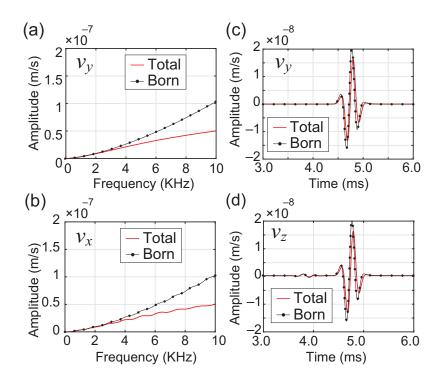
Figure C-2: Born approximated response (Born) and true response (Total) for zero-offset record in the configuration of Figure 4a. (a),(b) Modeled Green's functions for SH wavefield  $(v_y)$  and P-SV wavefield  $(v_x)$ . (c),(d) Time-domain responses of (a),(b) after convolution of Ricker wavelet with 3 KHz center frequency.
