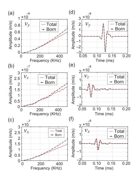
Figure C-1: Born approximated response (Born) and true response (Total) for zero-offset record in the configuration of Figure 1a. (a),(b),(c) Modeled Green's functions for SH wave-field  $(v_y)$  and P-SV wavefield  $(v_z)$  and  $v_x$ . (d),(e),(f) Time-domain responses of (a),(b),(c) after convolution of Ricker wavelet with 50 KHz center frequency.
