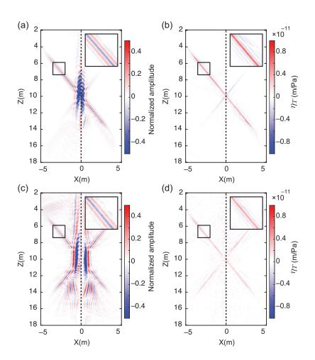
Figure 5: Imaging results using SH wavefield in dipole acoustic logging data; (a) Initial gradient without inversion, (b) the proposed LSM. (c),(d) Same as (a),(b) but using P-SV wavefield.
