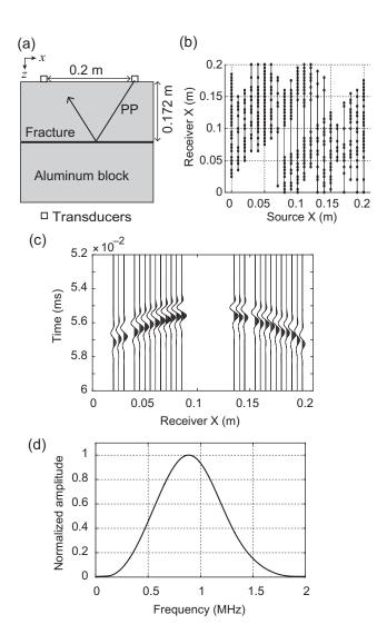
Figure 6: (a) Configuration of laboratory experiments. The fracture aperture is created using 100  $\mu$ m thick spacers. (b) Source–receiver geometry for the measured data. (c) An example of the measured PP reflection data for a source located at 0.11 m. (d) Frequency spectrum of (c).
