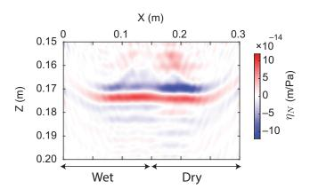
Figure 9: Imaging results on laboratory experimental data of a heterogeneously wet fracture using the proposed LSM (50–500 KHz).
