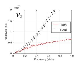
Figure 7: Frequency spectrum of the numerically modeled reflection response, representing the laboratory geometry and the fracture compliances. The total response and the Born approximation are shown.
