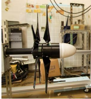
**Figure 1.2:** Dual-rotor configuration with both rotors placed behind the hub [11]
