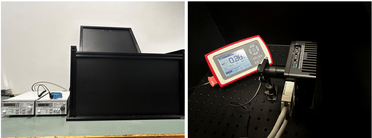
Figure 3.23: Left: Laser diode setup enclosed in a light-tight box to prevent ambient light interference. Right: Power measurement of the laser diode output using a photodetector.
