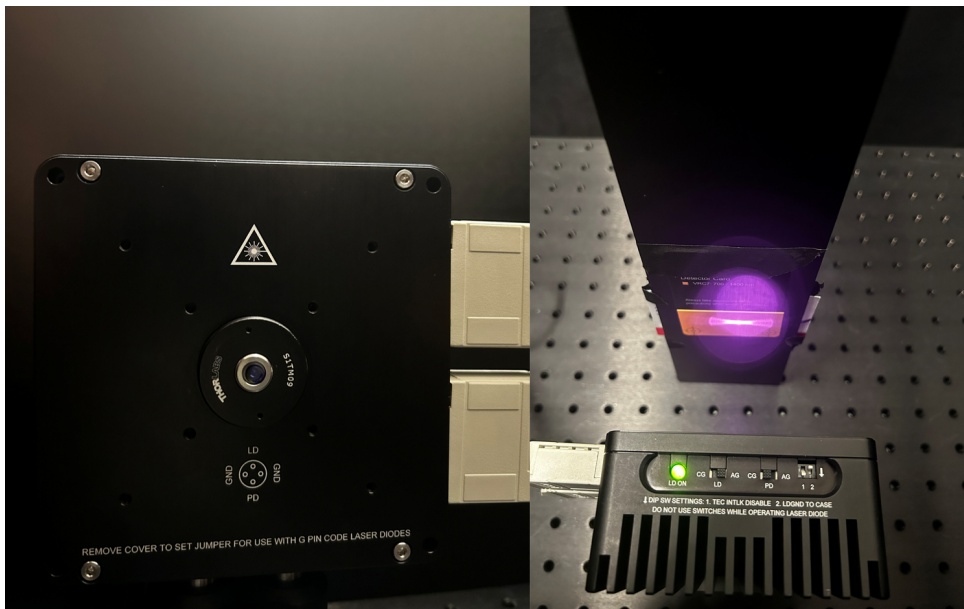
Figure 3.25: Collimating lens with laser diode structure and its light spot.
