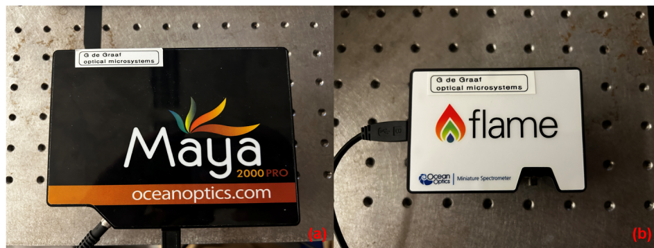
Figure 3.13: (a) Maya2000 Pro spectrometer can detect signals from 155–380nm. (b) FLAME spectrometer can detect signals from 360–1000nm
