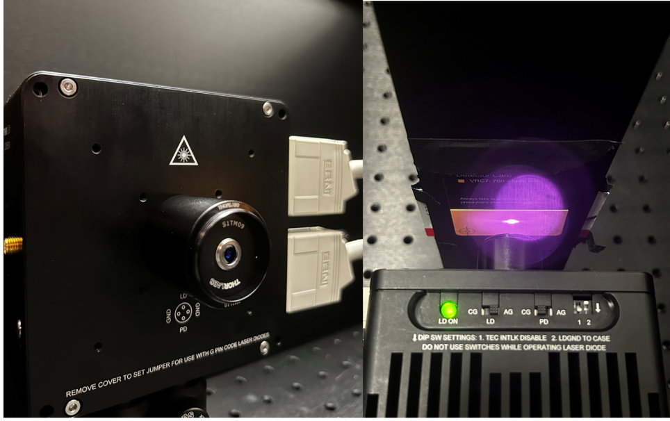
Figure 3.26: Focusing lens with laser diode structure and its light spot.
