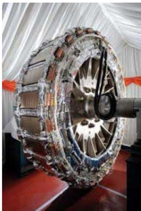
Figure 43 Full rotor assembly of the Hydrogenie generator
