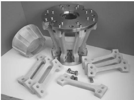
Figure 51 various parts of the torque tube during assembly
