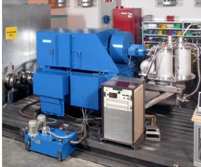
Figure 39 The Siemens 4 MVA HTS machine
