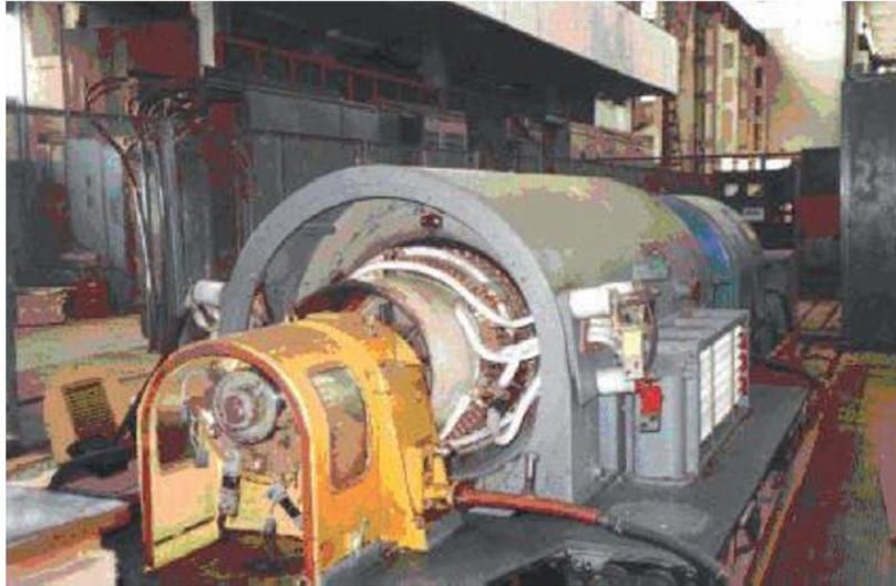
Figure 52 5 MVA 40 kV HTS synchronous generator
