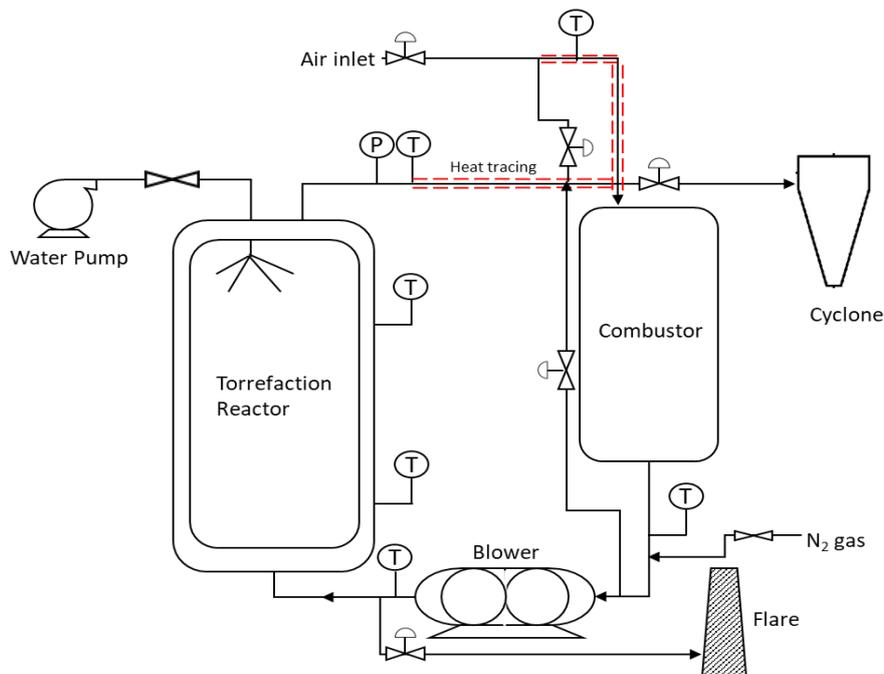
**Figure 6.** Torrefaction setup flowchart. Initially for drying, air enters from the top, is heated in the combustor and then led to the reactor. In torrefaction mode, the system closes to atmosphere, with the valve leading to the flare
