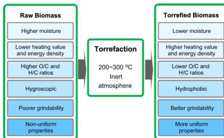
**Figure 1.** Main advantages of torrefaction on raw biomass's mechanical and thermochemical properties (W. H. Chen et al., 2015).
