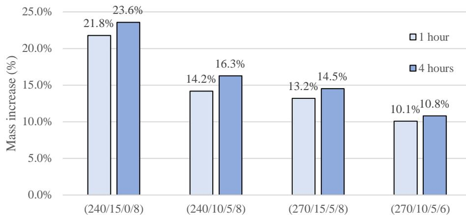
**Figure 16.** Moisture uptake for 4 different types of torrefied wheat straw pellets.
