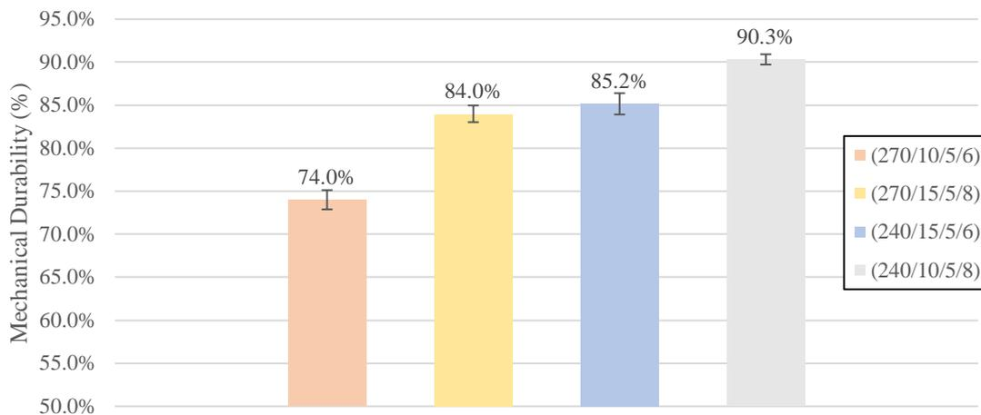
**Figure 14.** Mechanical durability results on the torrefied wheat straw pellets that contain plastic.
