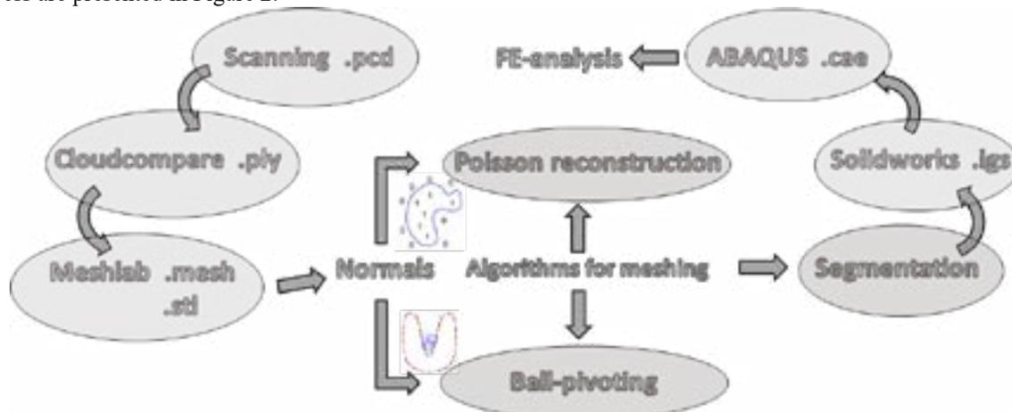
Figure 2: Flowchart, showing the process of the log reconstruction
