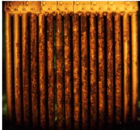
Figure 1.2: Corroded fuel rods at the Palo Verde Nuclear Generating Station. Figure from Walter et al. [4].
