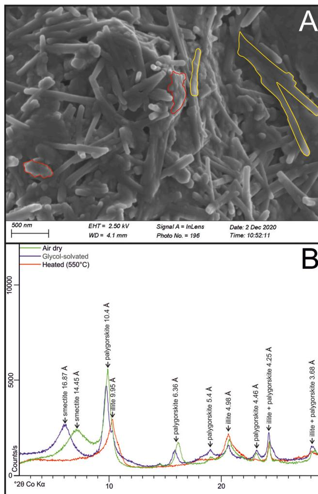
**Fig. 5.** A, BSE-imaging of palygorskite rods (highlighted in yellow) interspersed amongst fine-grained smectite (highlighted in red). B,  $<2 \mu\text{m}$  orientated clay X-ray diffraction scan showing principle low-angle palygorskite peaks.
