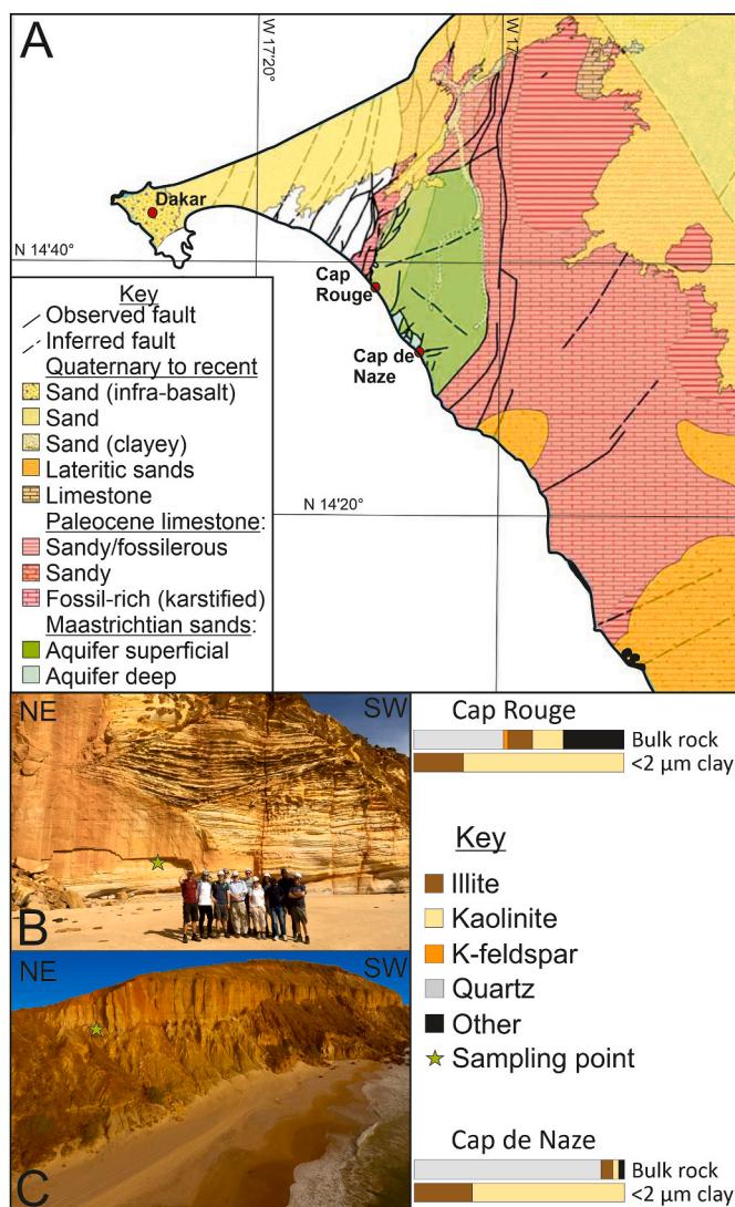
**Fig. 9.** A, Geological map of western Senegal (M'bour region) modified from Barusseau et al. (2009). B, Cap Rouge exposure and associated bulk rock and  $<2\text{ }\mu\text{m}$  clay mineralogy. C, Cap de Naze exposure and associated bulk rock and  $<2\text{ }\mu\text{m}$  clay mineralogy.
