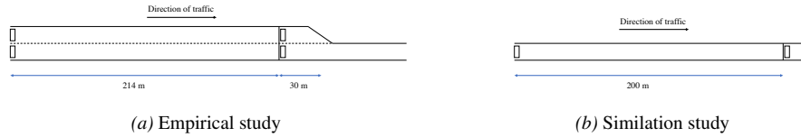
Figure 3.4: Lay-out of the on-ramps considered in the simulation and empirical case studies.
