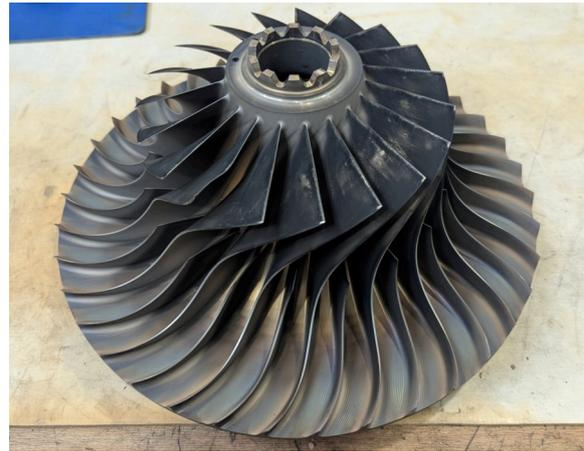
Figure 4.16: Used and unwashed impeller.
