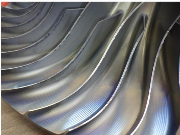
**Figure 3.6:** Impeller blade rubbing damage.
