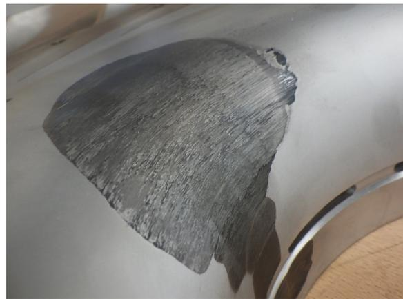
**Figure 3.7:** Shroud rubbing damage.
