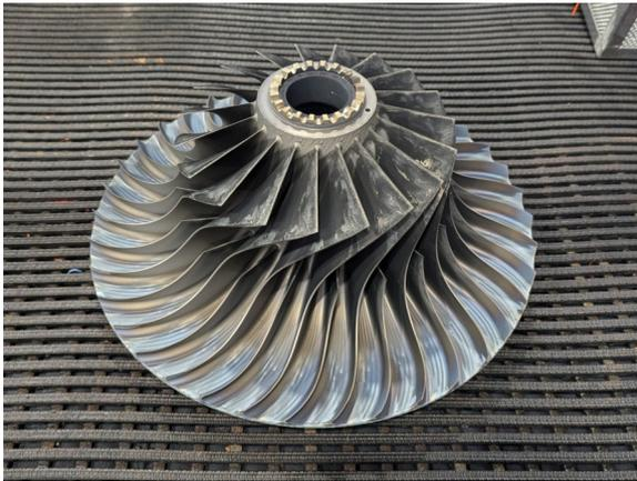
Figure 3.2: Compressor impeller.
