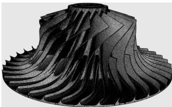
**Figure 4.1:** High fidelity impeller 3D scan.
