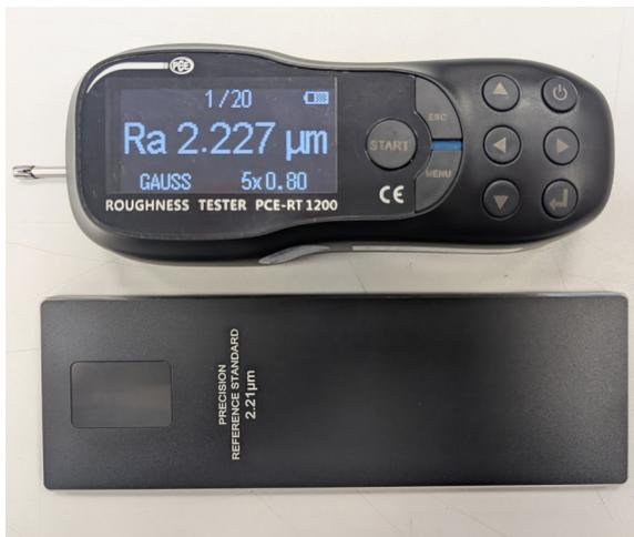
Figure 4.17: PCE-RT 1200 profilometer and calibration plate..
