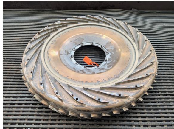
Figure 3.3: Compressor diffuser with exit guide vanes.
