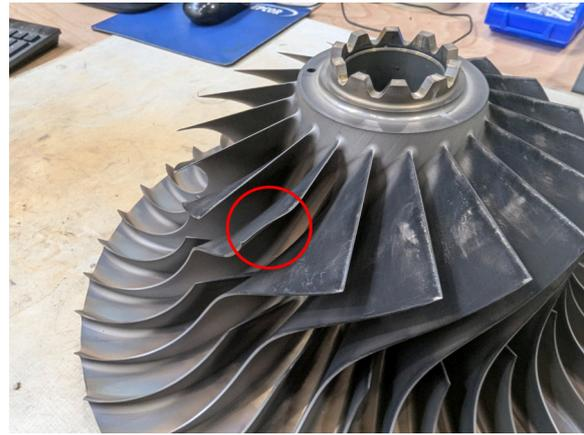
**Figure 3.5:** Impeller blade deformation marked by red circle.
