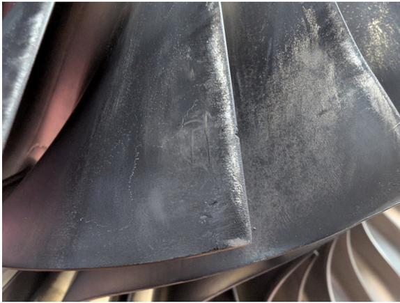
**Figure 3.4:** Impeller leading edge blade chipping and fouling.
