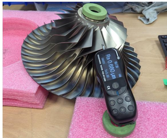
Figure 4.18: Surface roughness measurement close to leading edge of impeller..
