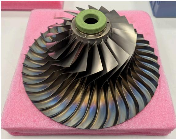
Figure 4.15: Within specification cleaned impeller.
