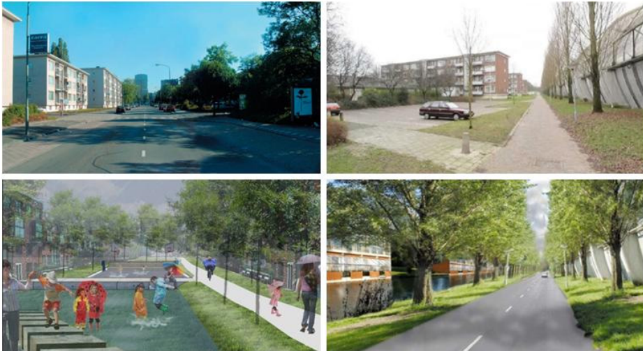
Figure 6.10. Illustration of the options selected for the minor/major system (bottom left) and open water system (bottom right). To clarify: (i) the bottom left figure shows the modified design for the park zone, which comprises a lowering of the green space to allow for temporary surface storage; (ii) the bottom right figure shows the design for the new open watercourse; (iii) the top photos represent the current situation at the two locations
