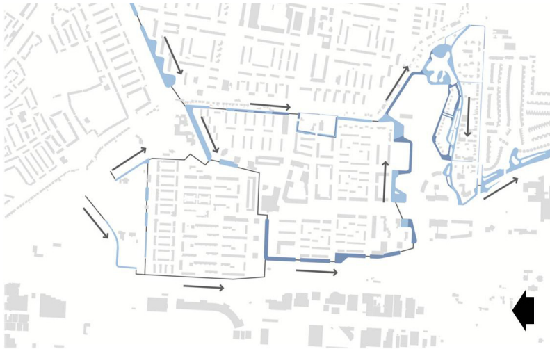
Figure 6.3. Layout of the open water system; light grey lines represent the current situation and dark grey lines represent the future situation after the regeneration project has been implemented
