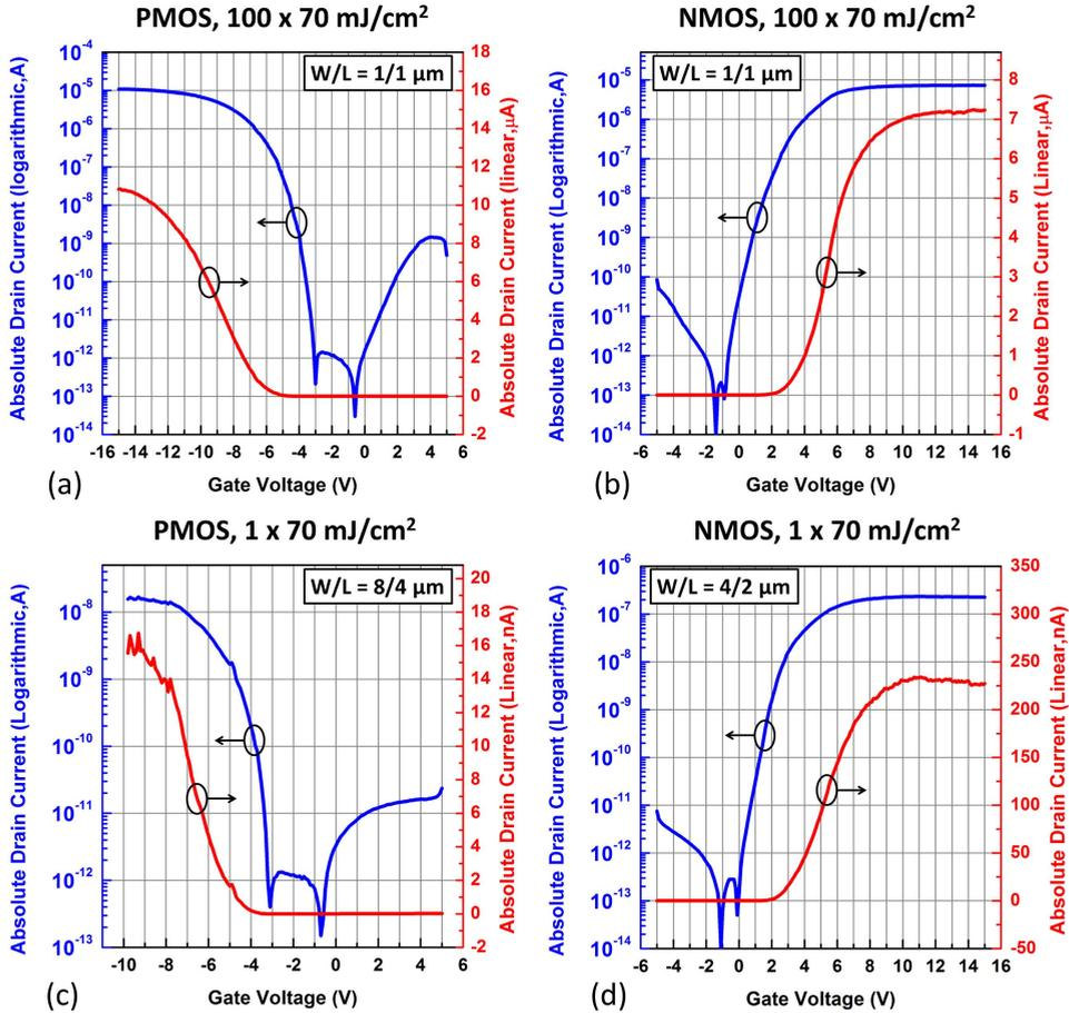
Figure 5.6: Transfer curves in linear (red) and logarithmic (blue) scale of 100 pulses of 70  $\text{mJ}/\text{cm}^2$  crystallized PMOS (a), NMOS (b), and single pulse of 70  $\text{mJ}/\text{cm}^2$  crystallized PMOS (c) and NMOS (d) TFTs.
