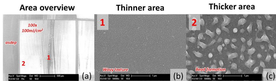
Figure 3.19: SEM images of an area exposed to 100 pulses of  $100 \text{ mJ}/\text{cm}^2$ . General overview of the area defining the two areas with different thicknesses 1 and 2 (a). Zoomed area of thickness 1 (b), and zoomed area of thickness 2 (c).
