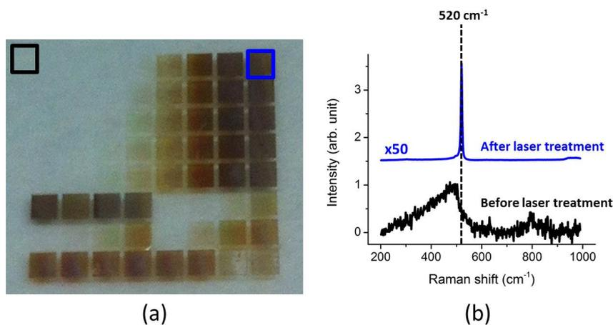
Figure 3.9: Optical image of polysilane cured with a UV intensity of  $10 \text{ mW/cm}^2$ , exposed to various excimer laser energy densities (a). Raman spectrum of one of the exposed areas and a non-exposed area (b).
