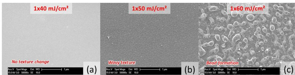
Figure 3.15: SEM image of single KrF ELA pulses at 40 mJ/cm<sup>2</sup> (a), 50 mJ/cm<sup>2</sup> (b), 60 mJ/cm<sup>2</sup> (c).
