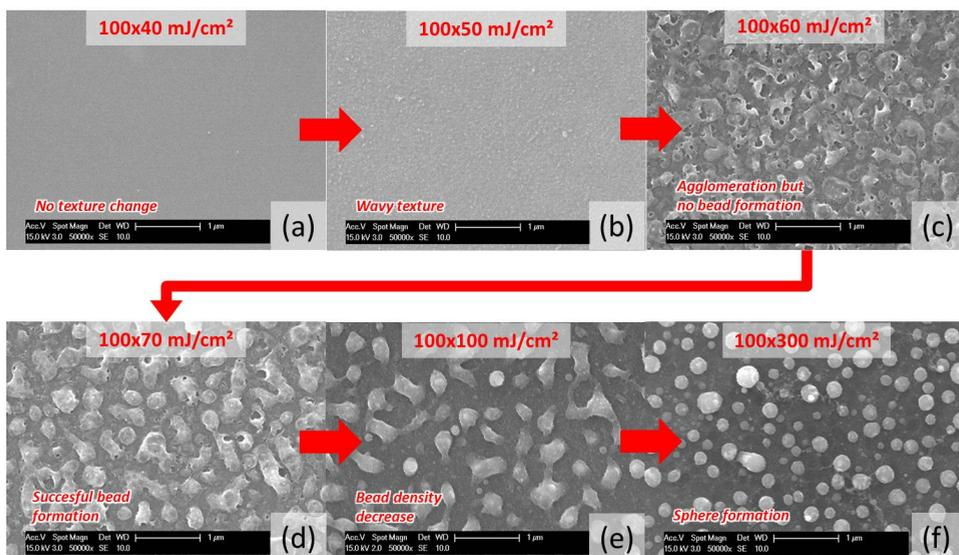
Figure 3.16: SEM image of 100 KrF ELA pulses per energy density area: 40 mJ/cm<sup>2</sup> (a), 50 mJ/cm<sup>2</sup> (b), 60 mJ/cm<sup>2</sup> (c), 70 mJ/cm<sup>2</sup> (d), 100 mJ/cm<sup>2</sup> (e), 300 mJ/cm<sup>2</sup> (f).
