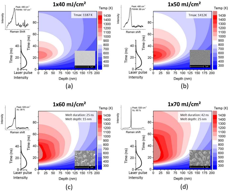
Figure 4.7: Transient heat simulation results of 200 nm polysilane exposed to a single KrF laser pulse with various energy densities: 40 mJ/cm<sup>2</sup> (a), 50 mJ/cm<sup>2</sup> (b), 60 mJ/cm<sup>2</sup> (c), 70 mJ/cm<sup>2</sup> (d). All samples have an associated SEM image and Raman measurement obtained from experimental data.
