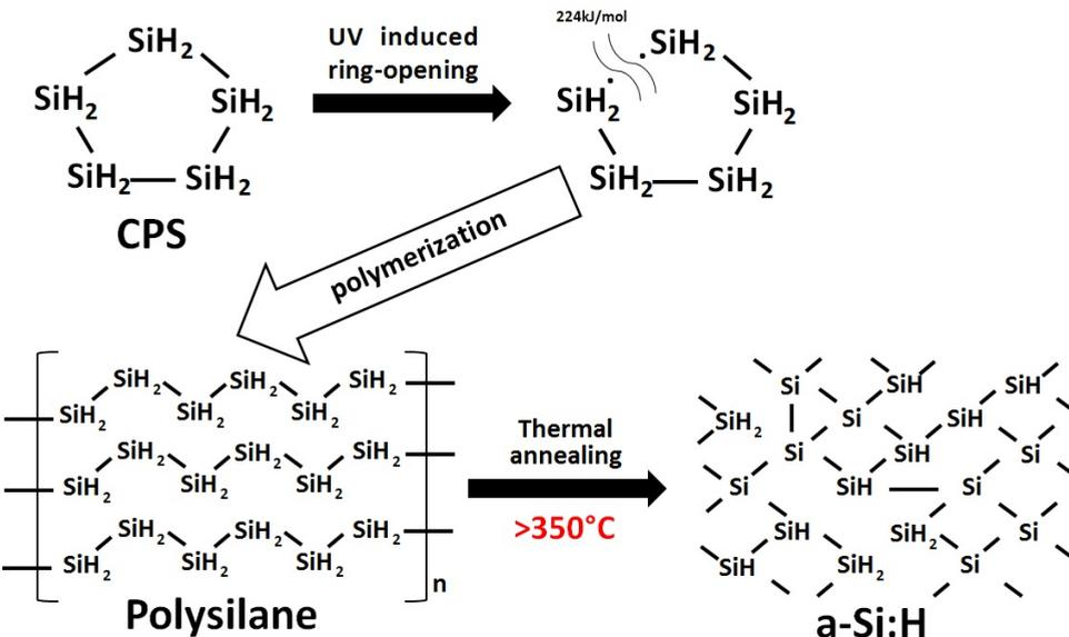
Figure 2.3: Transformation process from CPS to a-Si:H.
