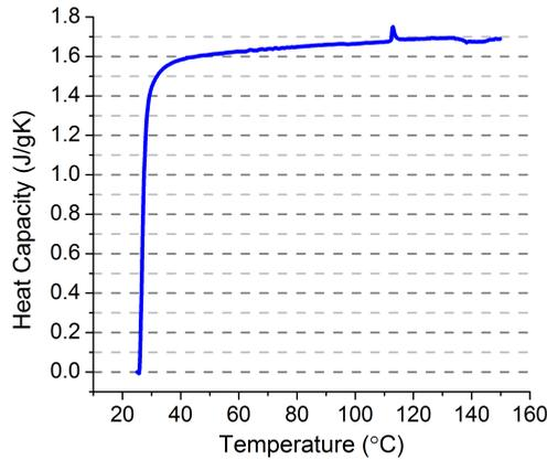
Figure 4.6: Differential scanning calorimetry measurements of polysilane.
