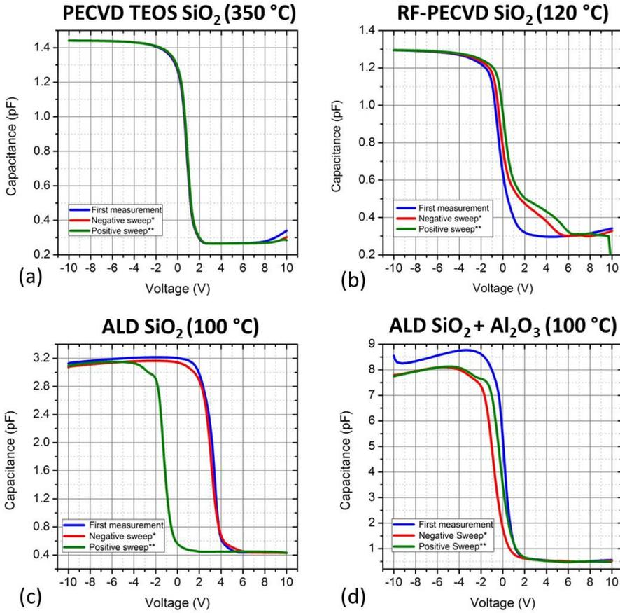
Figure 5.3: Capacitance to voltage measurements for four different types of oxides: PECVD TEOS SiO<sub>2</sub> (a), RF-PECVD SiO<sub>2</sub> (b), ALD SiO<sub>2</sub> (c), ALD SiO<sub>2</sub> + Al<sub>2</sub>O<sub>3</sub> (d). Each displaying three curves: first measurement (blue), repeated measurements (red), and opposite voltage sweep (green).
