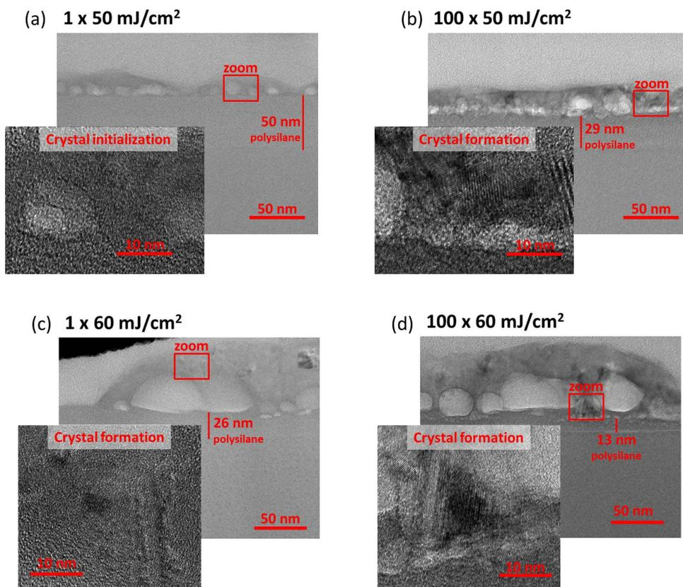
Figure 3.14: Cross-sectional TEM images of polysilane exposed to a KrF laser with different treatments:  $1 \times 50 \text{ mJ/cm}^2$  (a),  $100 \times 50 \text{ mJ/cm}^2$  (b),  $1 \times 60 \text{ mJ/cm}^2$  (c), and  $100 \times 60 \text{ mJ/cm}^2$  (d).
