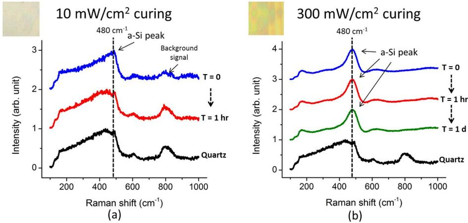
Figure 3.5: Raman spectra of CPS cured with 10 mW/cm<sup>2</sup> (a), and 300 mW/cm<sup>2</sup> (b).
