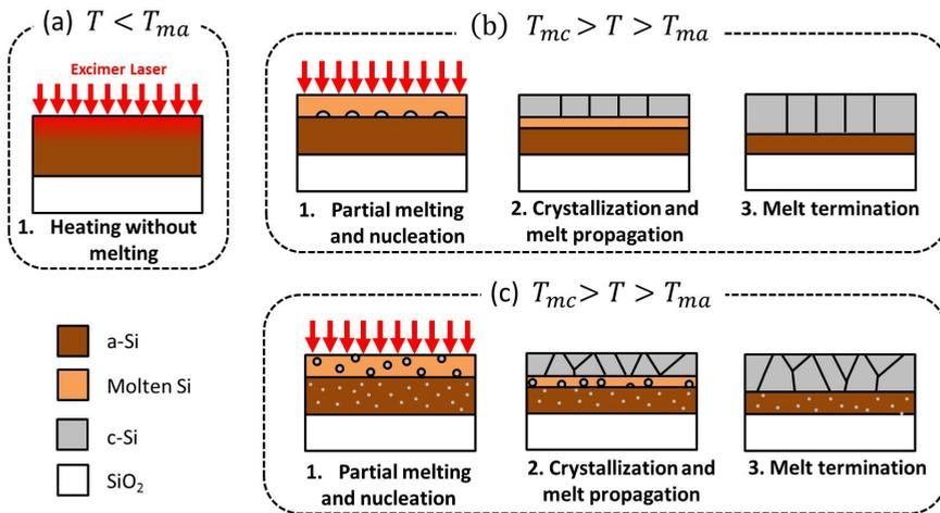
Figure 4.2: Schematic of excimer laser annealing where film reaches temperature below  $T_{ma}$  (a), between  $T_{ma}$  and  $T_{mc}$  for pure a-Si (b), and between  $T_{ma}$  and  $T_{mc}$  for a-Si with crystalline fraction (c).
