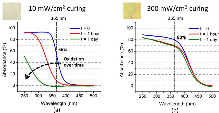
Figure 3.6: Absorption spectra of CPS samples cured with 10 mW/cm<sup>2</sup> (a) and 300 mW/cm<sup>2</sup> (b).
