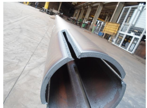
Figure 2.4: Example of a cut by an HGG PE machine [10]
