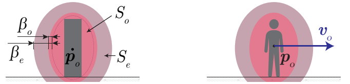
Fig. 2: Cuboid obstacle (left) with fixed position \mathbf{p}_o or dynamic (human) obstacle (right) with constant velocity \mathbf{v}_o each modelled by bounding S_o and expanded S_e ellipsoid with dimensional buffers \beta .
