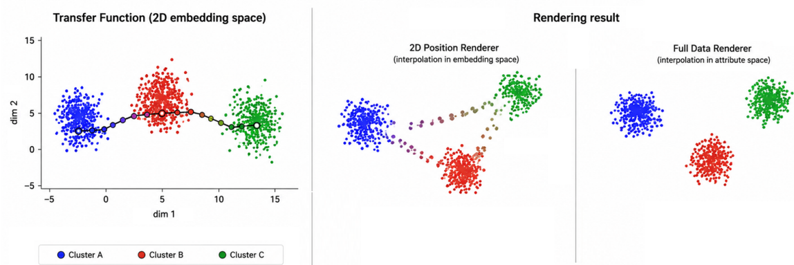
Figure 4.4: Illustration of interpolation artifacts in the 2D position renderer. The left image shows a TF defined in a 2D embedding space with three separated clusters. The middle image shows the result of interpolating directly between embedding positions, as done by the 2D position renderer. This interpolation can create artificial intermediate positions between unrelated clusters, which may lead to incorrect color and opacity values. The right image shows the full data renderer, where interpolation is performed in the original attribute space before mapping the sample to the embedding. This better preserves the intended separation between structures.
