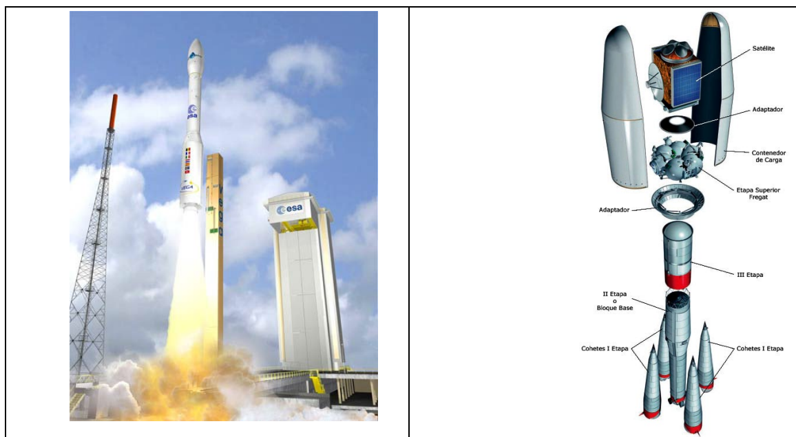
Figure 9: Vega (left) and Soyuz rocket exploded view (right) (courtesy ESA)
