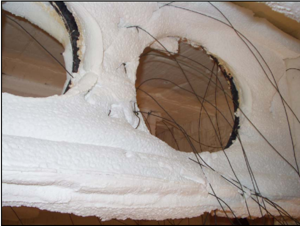
Figure 2.25 Swelling of intumescent coating due to fire
