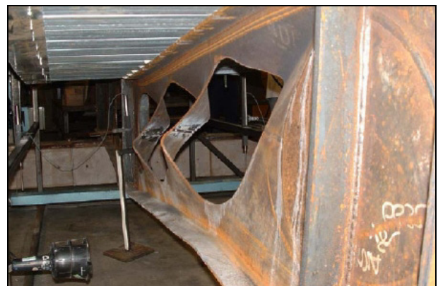
Figure 3.7 Web-post lateral-torsional buckling due to (vertical) shear
