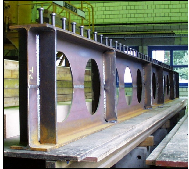
Figure 2.8 Web-post stiffeners and headed studs for composite application
