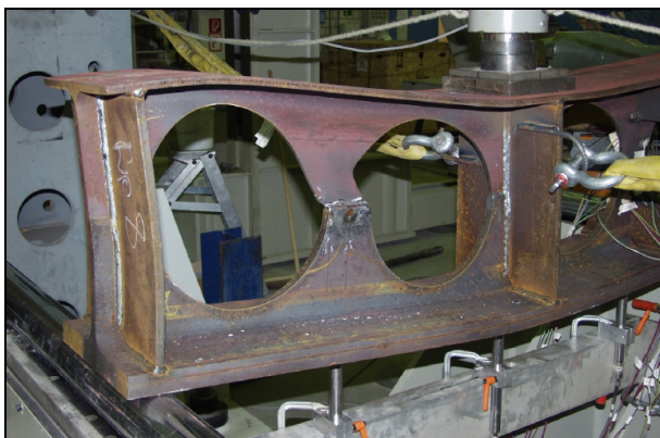
Figure 3.4 Web-post yielding due to horizontal shear
