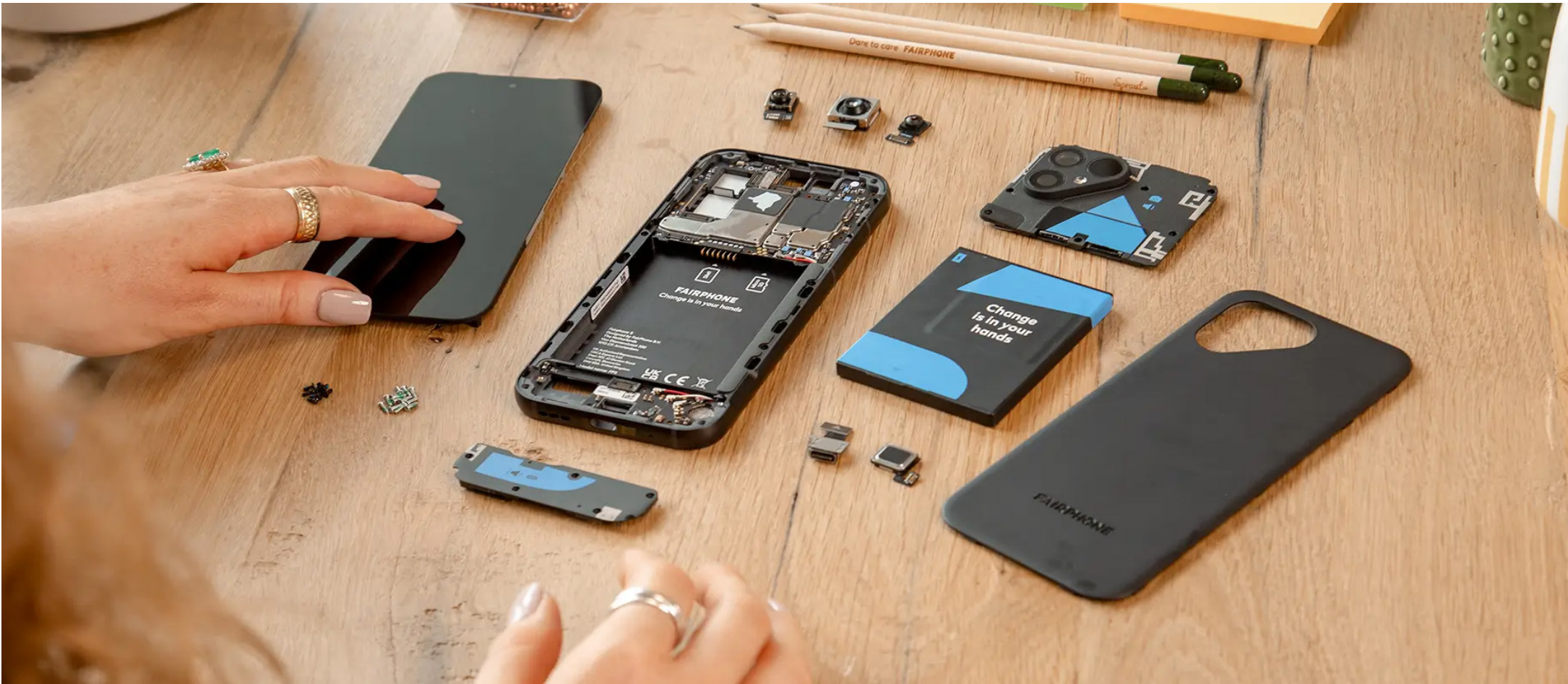
Figure 8. The Fairphone 5, a modular smartphone and example of Design of Ease of Maintenance and Repair (Fairphone, 2023)
