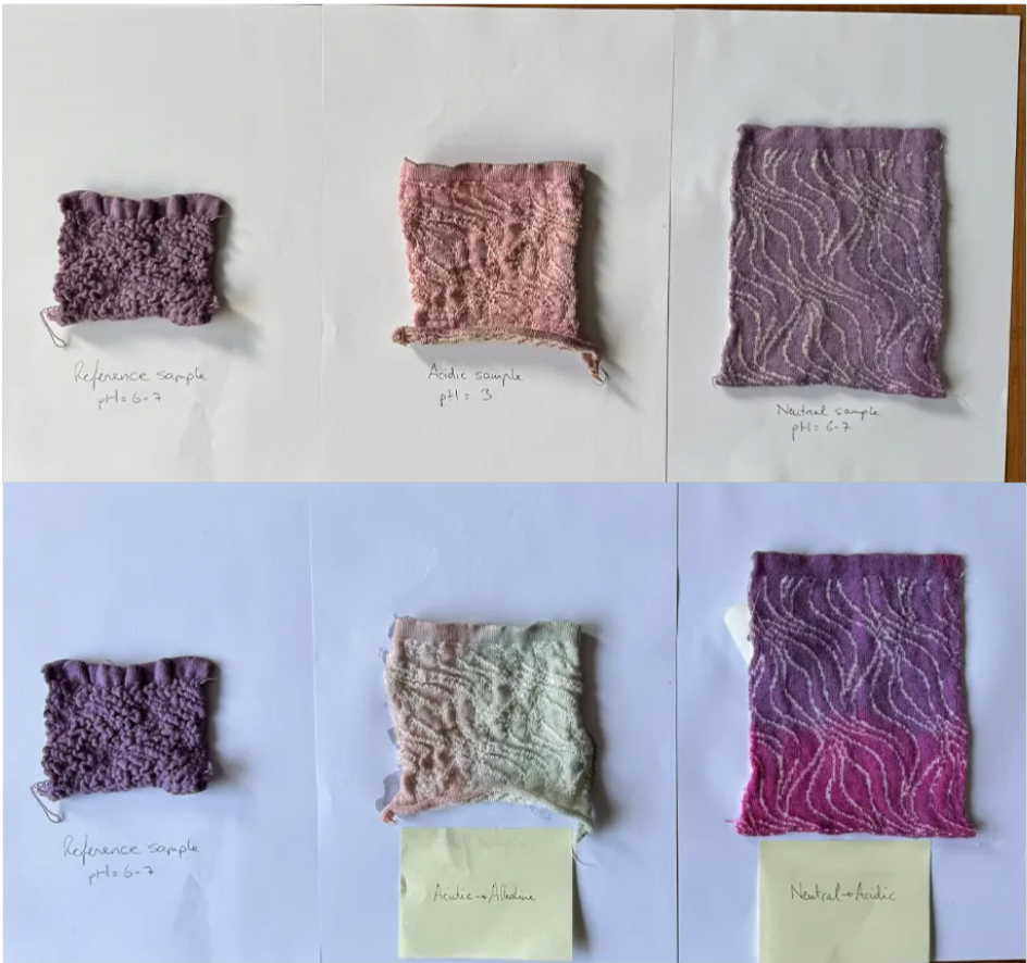
Figure 58. Samples before and after colour change. Fabricated by Rebekka Groeneveld and dyed by Stefano Parisi, IDE TU Delft.
