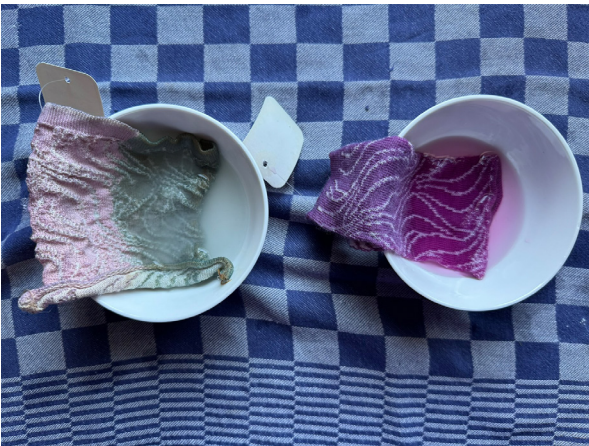
Figure 59. Samples portraying halochromism when dipped in alkaline (left) and acidic (right) solutions.
