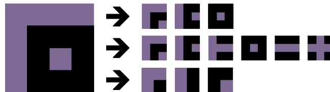
FIGURE 3.16: 3x3—sized patterns extracted without (top) and with (middle) input wrapping; 2x2—sized patterns (bottom). (Input image: SimpleMaze [11] with adapted colours)
