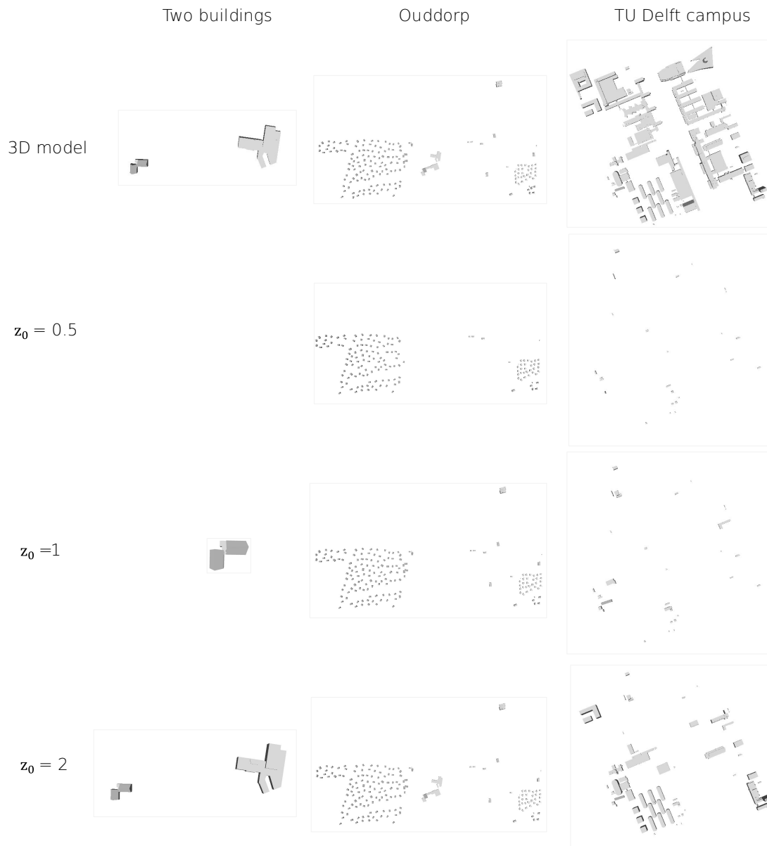
Figure 5.31.: Number of buildings with less than 10 cells per cube root building volume ( \sqrt[3]{\text{building volume}} ) within real-world datasets.
