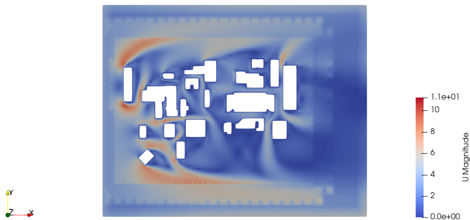
Figure 5.38.: Slide at 5m of CFD simulation with mesh parameters from tutorial.
