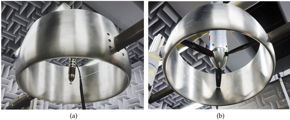
Figure 6.2: The omni-directional source (a) and the propeller (b) positioned in the center of the duct.
