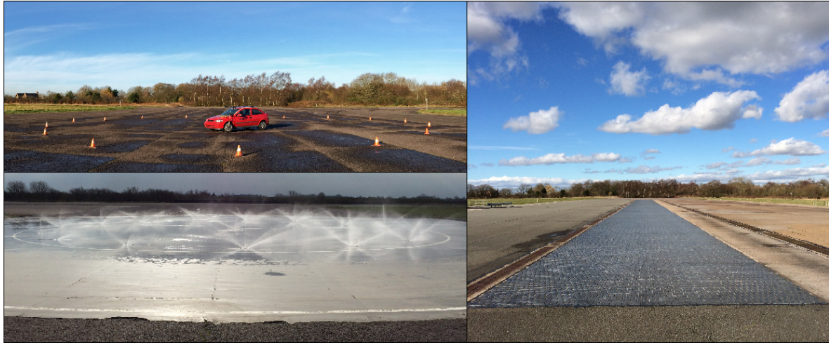
Figure 2-5: Prodrive test track: high and low \mu circles and straights
