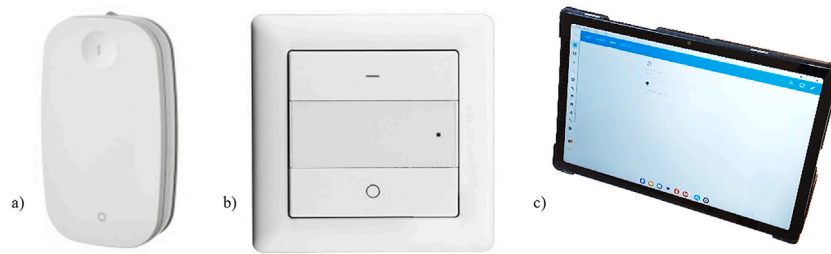
Fig. 4. Types of device interfaces used in the experiment: (a) analog light switch, (b) analog roller shade switch, and (c) tablet interface controlling both lights and roller shades.
