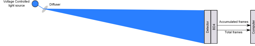
Figure 6.6: Frame accumulation at varying light intensity setup
