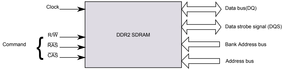
Figure 3.1: DDR2 block diagram
