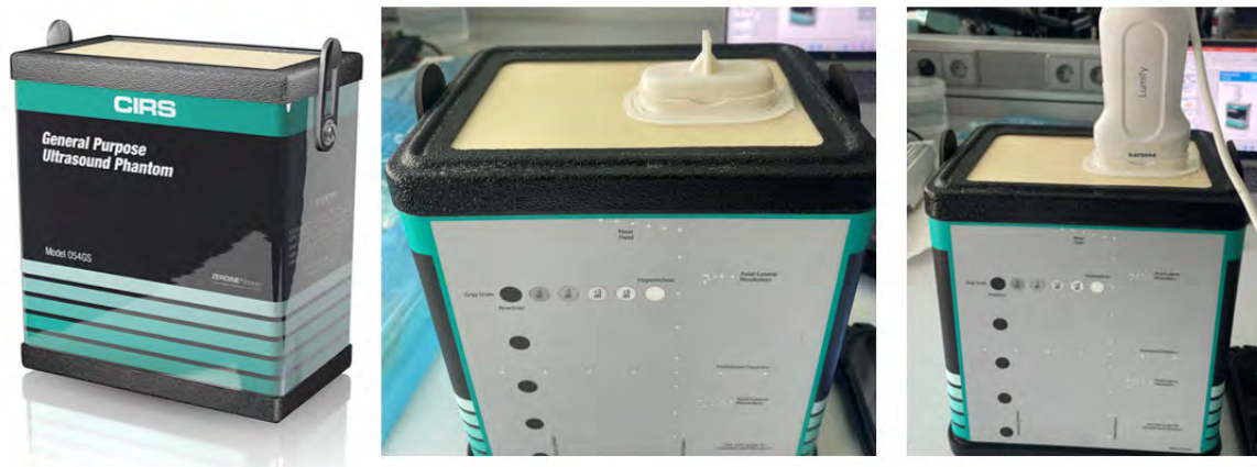
Figure 4.5: Images of CIRS General Purpose Ultrasound Phantom. Left: image acquired from: datasheet [56]. Middle: ultrasound phantom with 3D printed wearable ultrasound patch and pod on top. Right: ultrasound phantom with 3D printed wearable ultrasound patch with Philips Lumify clicked in.
