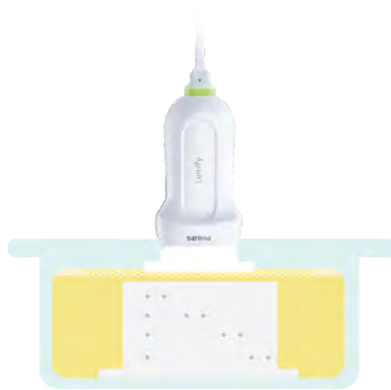
Figure 6.14: Schematic illustration of an ultrasound transducer on a phantom model. It illustrates how the ultrasound images were made during the lifetime experiments for testing performances of acoustic interface materials
