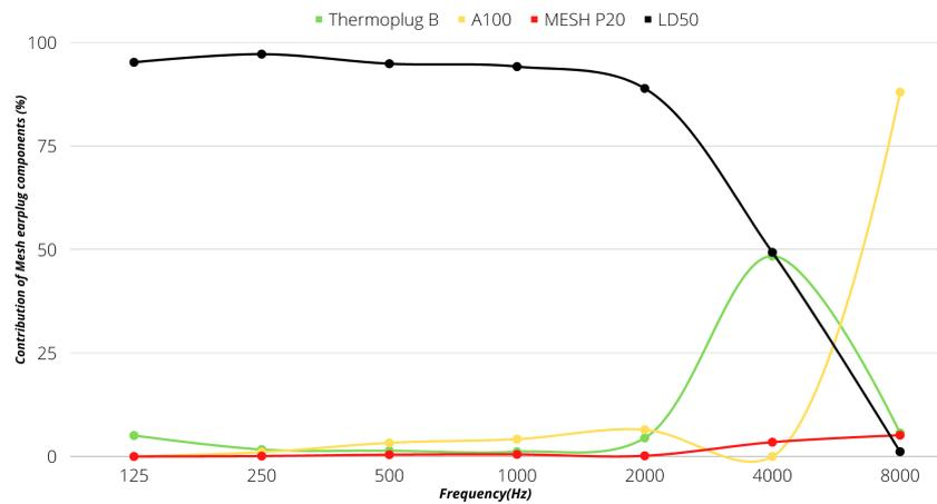
(b) Contribution of Thermoplug, Layer 1 - A100, Layer 2 - Mesh filter P20 and Layer 3 - LD50 in Product 4
