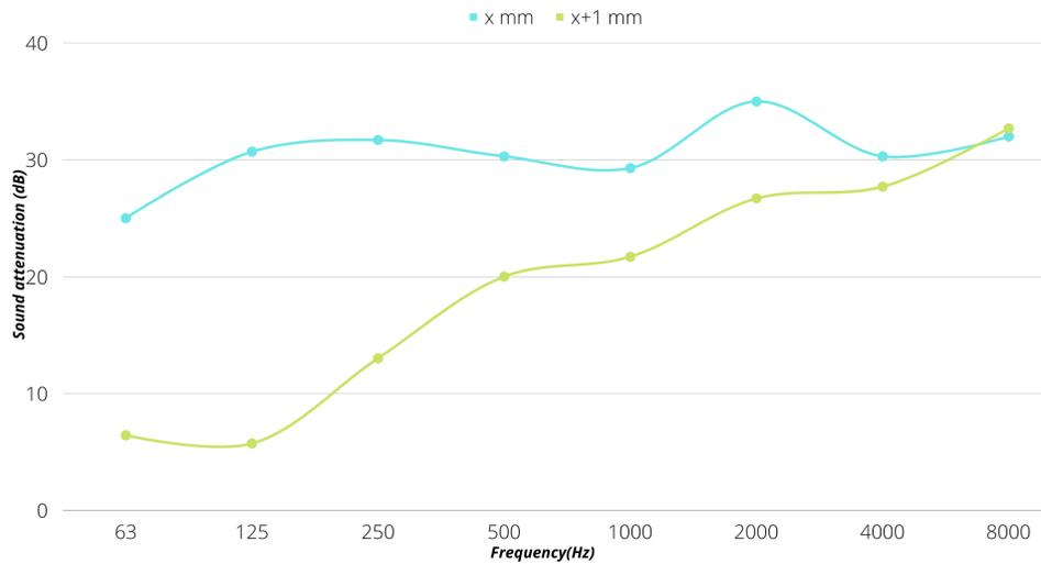
(a) Plot of Frequency (Hz) vs Sound Attenuation (dB) for different thermoplug canal length  $x$  mm (Blue curve),  $x+1$  mm (Green curve) of two different subjects. The plot shows that the attenuation decreases with an increase in the thermoplug canal diameter
