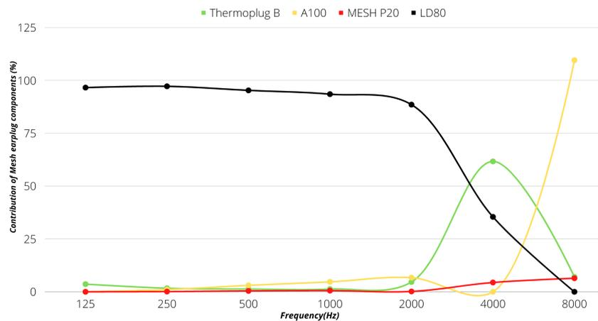
(c) Contribution of Thermoplug, Layer 1 - A100, Layer 2 - Mesh filter P20 and Layer 3 - LD80 in Product 5
