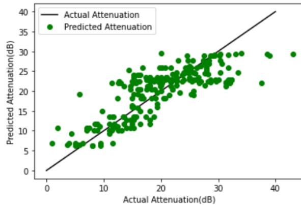
**Figure 4.1:** Actual Attenuation values (Black line) vs Predicted Attenuation values (Green dots) of venturi dataset with MAE of 3.5
