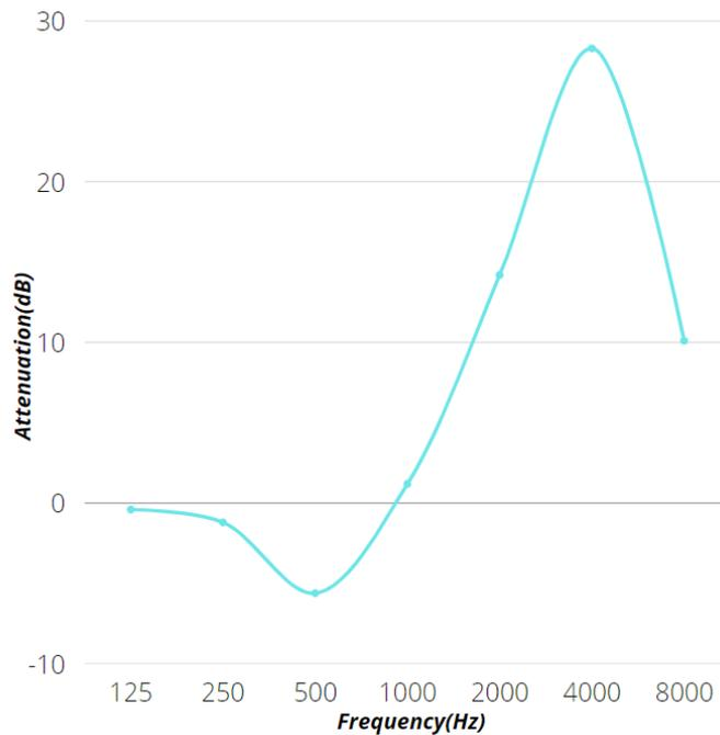
**Figure 2.4:** This graph shows the sound attenuation provided by the thermoplug component produced by the company ALPINE [4]. The thermoplug is tested without any filter inserted inside it (just an open area filled with air). The x-axis denotes the frequency in Hz and y-axis denotes the attenuation level in dB. It is observed that the thermoplug itself provides some sound dampening between 1000 - 4000 Hz
