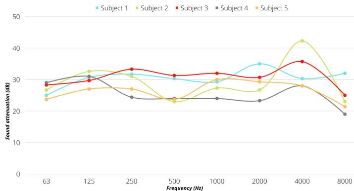
**Figure 3.17:** Frequency (Hz) vs Attenuation (dB) plot for first five subjects of Product 1 in soft filter Range. The same product, tested on different subjects results in different attenuation values for each frequency
