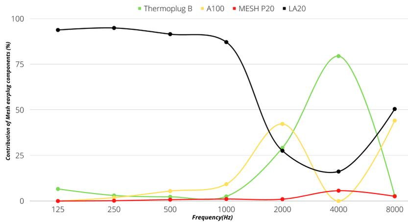
(b) Contribution of Thermoplug (Green curve), Layer 1 - A100 (Yellow curve), Layer 2 - Mesh filter P20 (Red curve) and Layer 3 - LA20 (Black curve) in Product 8. The x-axis is the frequency in Hz and y-axis is the contribution of mesh earplug components in %. Like Product 7, in low frequencies layer 3 - LA20 contributes the most and at 4000 Hz, thermoplug contributes the most. However, at 8000 Hz, contribution of layer 3 - LA20 is better than Layer 1 - A100.
