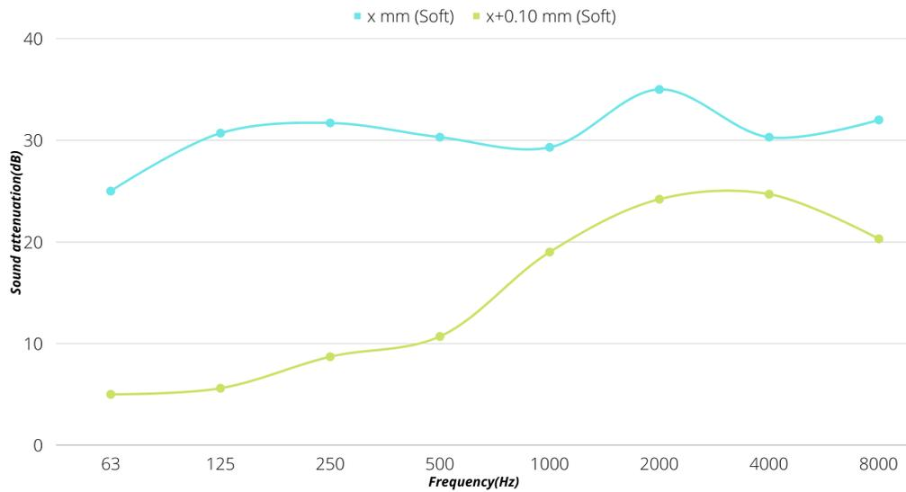
(a) Plot of Frequency (Hz) vs Attenuation (dB) for different filter diameters  $x$  mm (Blue curve) and  $x+0.10$  mm (Green curve) of two different subjects in soft range filters
