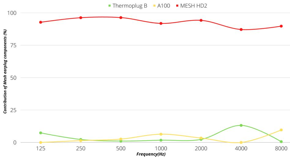
(b) Contribution of Thermoplug (Green curve), Layer 1 - A100 (Yellow curve), and Layer 2 - Mesh filter HD2 (Red curve) in Product 10. The x-axis is the frequency in Hz and y-axis is the contribution of mesh earplug components in %. Most of the contribution to total attenuation is from the mesh filter
