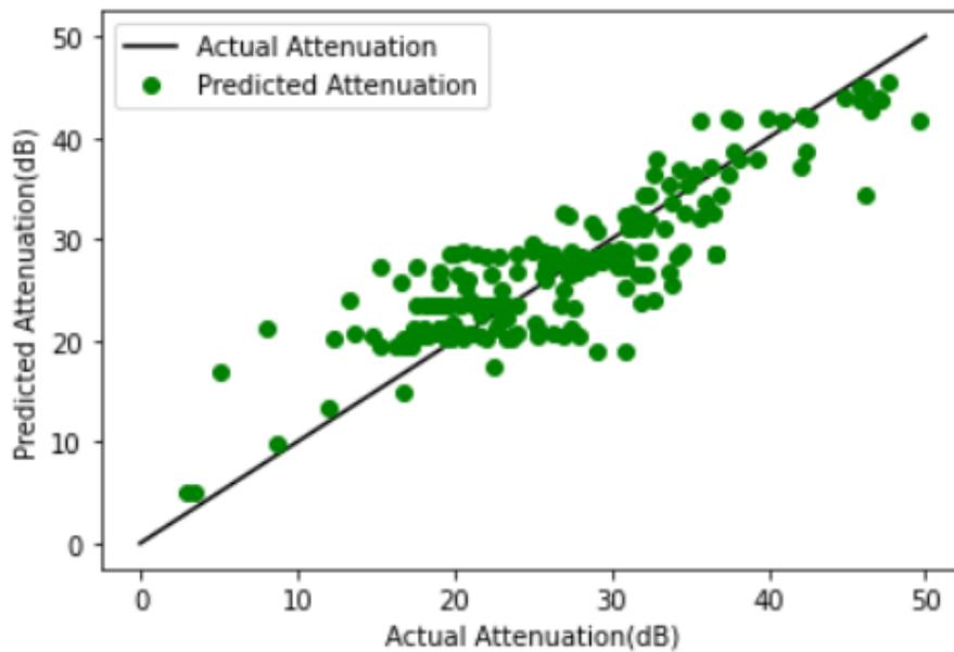
**Figure 4.6:** Actual Attenuation values (Black line) vs Predicted Attenuation values (Green dots) of mesh dataset with MAE of 3.26
