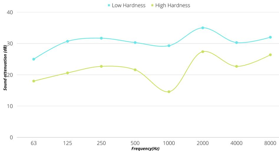
(b) Plot of Frequency(Hz) vs Sound Attenuation(dB) for low (Blue curve) and high (Green curve) filter Hardness of two different subjects. From the plot it is clear that the material with low hardness has better attenuation than a material with high hardness
