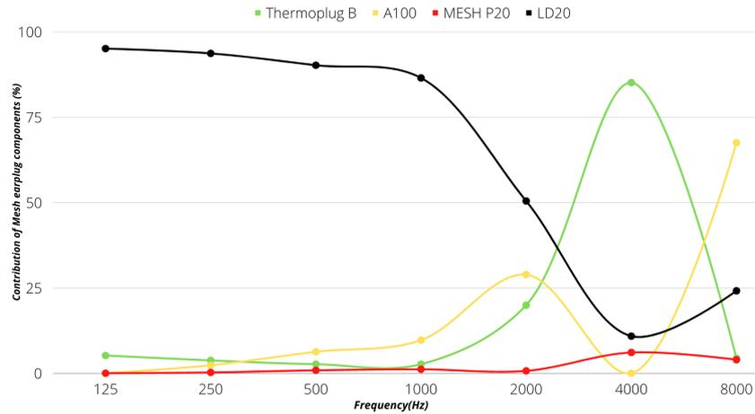
(a) Contribution of Thermoplug, Layer 1 - A100, Layer 2 - Mesh filter P20 and Layer 3 - LD20 in Product 3
