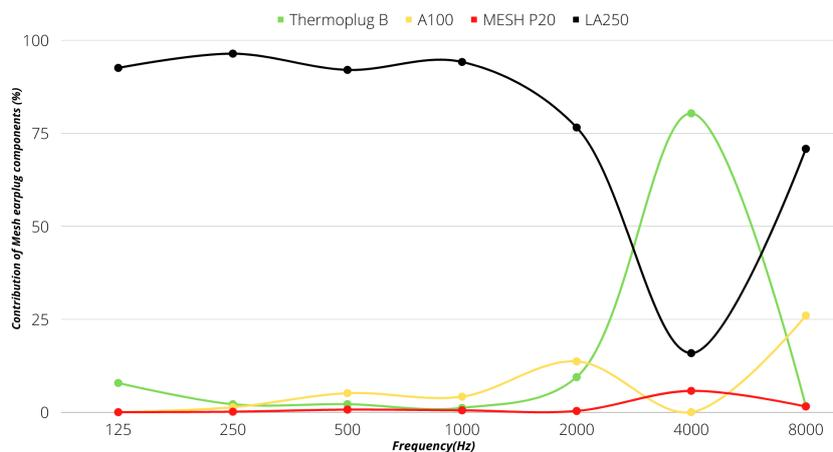
(c) Contribution of Thermoplug (Green curve), Layer 1 - A100 (Yellow curve), Layer 2 - Mesh filter P20 (Red curve) and Layer 3 - LA250 (Black curve) in Product 9. The x-axis is the frequency in Hz and y-axis is the contribution of mesh earplug components in %. Like Product 7 and 8, in low frequencies layer 3 - LA250 contributes the most and at 4000 Hz, thermoplug contributes the most. At 8000 Hz, Layer 3 - LA250 contributes the most.
