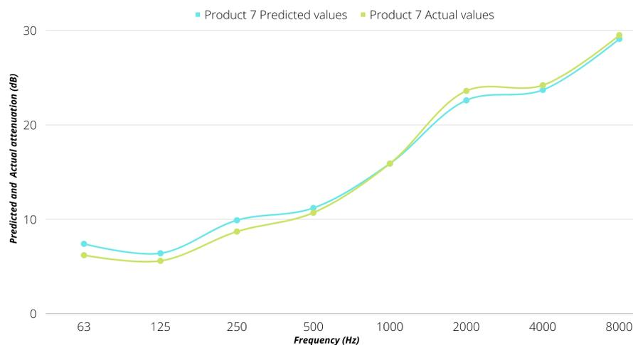
**Figure 4.4:** Comparison of predicted (Blue curve) and actual attenuation values (Green curve) in Product 7 (Hard Range Filter). The x-axis is the frequency in Hz and y-axis is the predicted (Blue curve) and actual (Green curve) sound attenuation in dB. The predicted values are almost the same as the actual values
