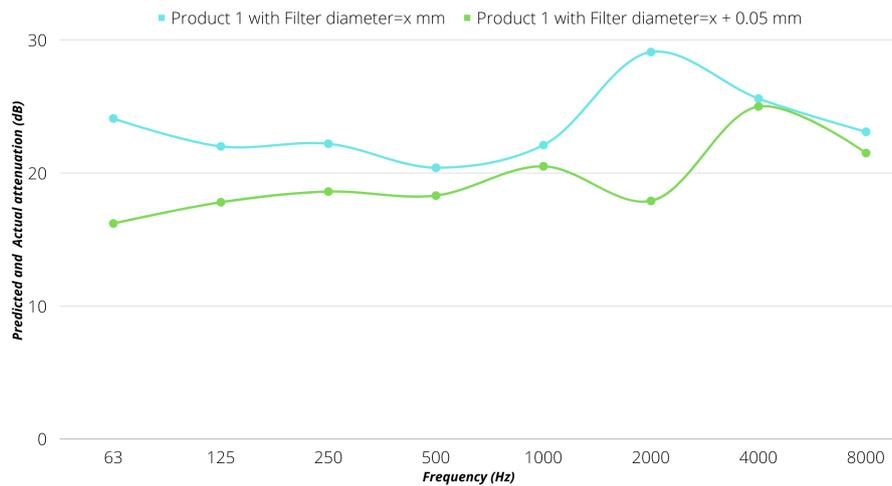
**Figure 4.5:** Comparison of predicted attenuation values for different filter diameters of x mm (Blue curve) and x+0.05 mm (Green curve). The x-axis is the frequency in Hz and y-axis is the predicted (Green curve) and actual (Blue curve) sound attenuation in dB. As the filter diameter increases the predicted attenuation decreases
