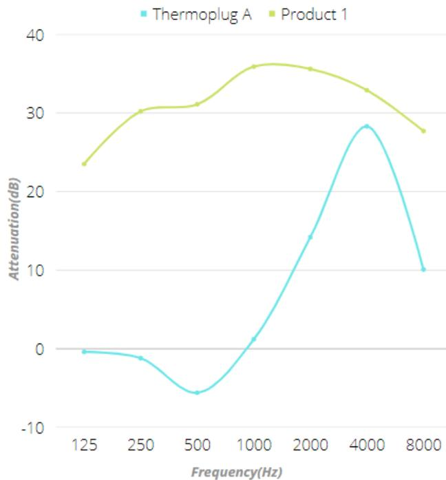
**Figure 3.8:** Sound attenuation provided by just the Thermoplug A (without filter) vs Sound attenuation provided by Product 1 (Thermoplug A with filter of x mm diameter). The x-axis is the frequency in Hz and y-axis is the sound attenuation in dB. The blue curve is the sound attenuation provided by the thermoplug A and the green curve is the sound attenuation provided by Product 1. Most of the attenuation in Product 1 is from the thermoplug at 4000 Hz
