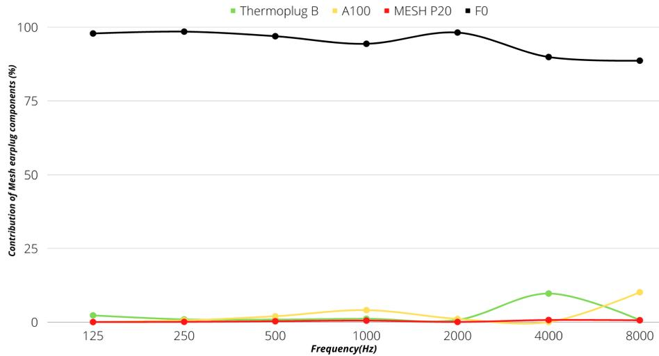
**Figure 3.12:** Contribution of Thermoplug (Green curve), Layer 1 - A100 (Yellow curve), Layer 2 - Mesh filter P20 (Red curve) and Layer 3 - FO (Black curve) in Product 6. The x-axis is the frequency in Hz and y-axis is the contribution of mesh earplug components in %. Most of the contribution to total attenuation IN Product 6 is from FO layer when compared to all other components
