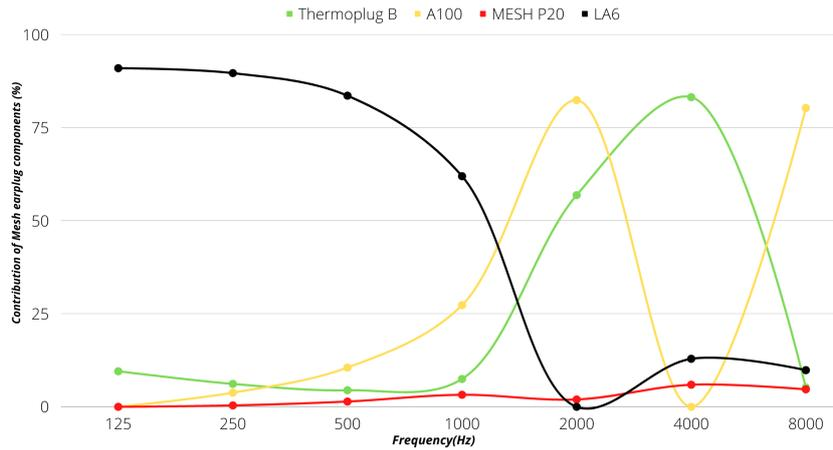
(a) Contribution of Thermoplug (Green curve), Layer 1 - A100 (Yellow curve), Layer 2 - Mesh filter P20 (Red curve) and Layer 3 - LA6 (Black curve) in Product 7. The x-axis is the frequency in Hz and y-axis is the contribution of mesh earplug components in %. In low frequencies layer 3 - LA6 contributes the most and at 4000 Hz, thermoplug contributes the most. However, at 2000 Hz and 8000 Hz, Layer 1 - A100 contributes the most
