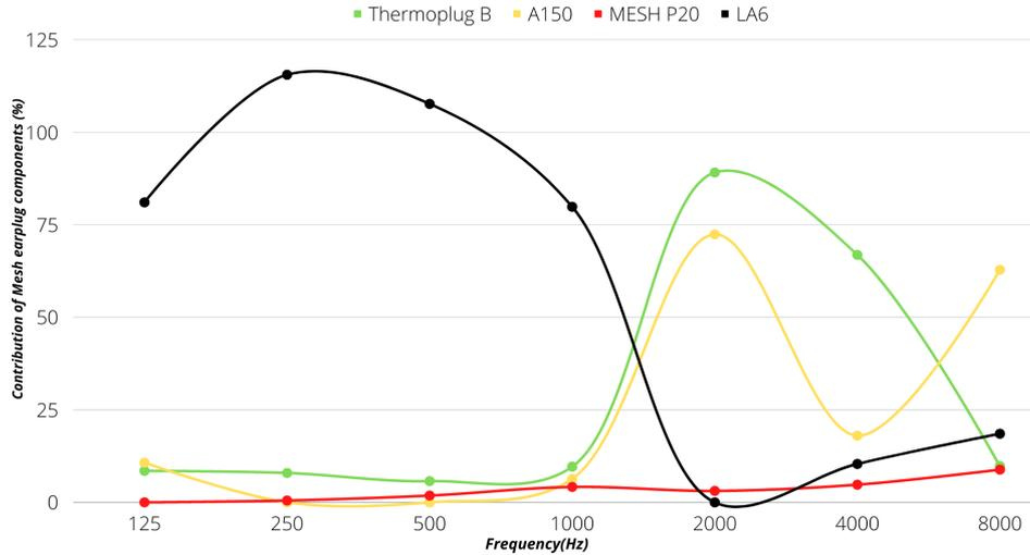
**Figure 3.15:** Contribution of Thermoplug (Green curve), Layer 1 -A150 (Yellow curve), Layer 2 - Mesh filter P20 (Red curve) and Layer 3 -LA6 (Black curve) in Product 12. The x-axis is the frequency in Hz and y-axis is the contribution of mesh earplug components in %. It is clear that at low frequencies, the contribution of layer 3 - LA6 is maximum. Around 4000 Hz, thermoplug contributes the most. Around 8000 Hz contribution of layer 1 - A150 is more than the other components
