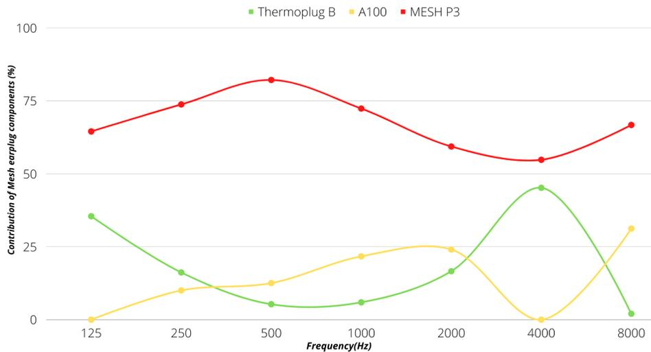
(a) Contribution of Thermoplug (Green curve), Layer 1 - A100 (Yellow curve), and Layer 2 - Mesh filter P3 (Red curve) in Product 10. The x-axis is the frequency in Hz and y-axis is the contribution of mesh earplug components in %. Most of the contribution to total attenuation is from the mesh filter
