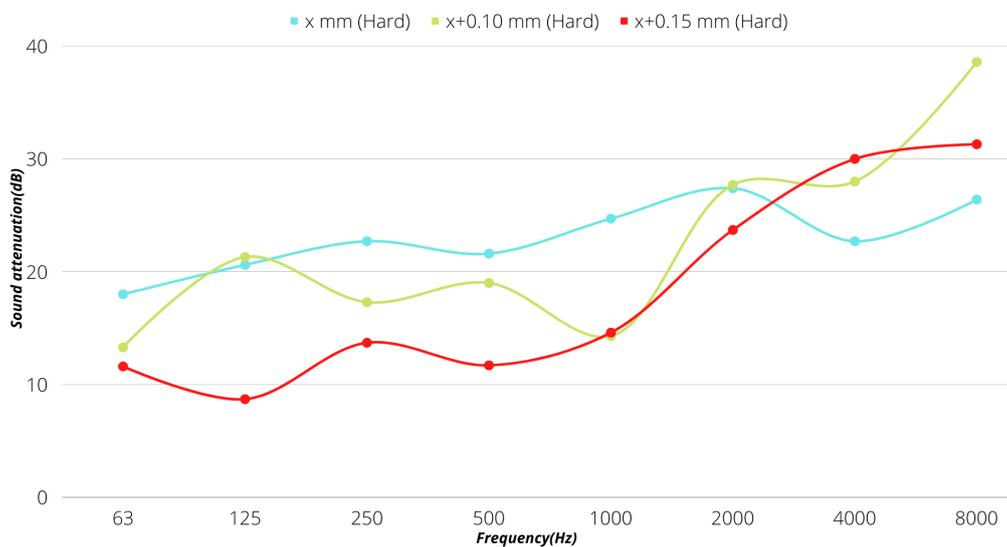
(b) Plot of Frequency (Hz) vs Attenuation (dB) for different filter diameters  $x$  mm (Blue curve),  $x+0.10$  mm (Green curve) and  $x+0.15$  mm (Red curve) of two different subjects in hard range filters
