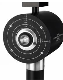
**Figure 2.2:** This figure shows the Acoustic Test Fixture with a microphone that measures the insertion loss by measuring the sound pressure level with and without the earplug. The earplug is inserted into the small circular opening in the middle [8].
