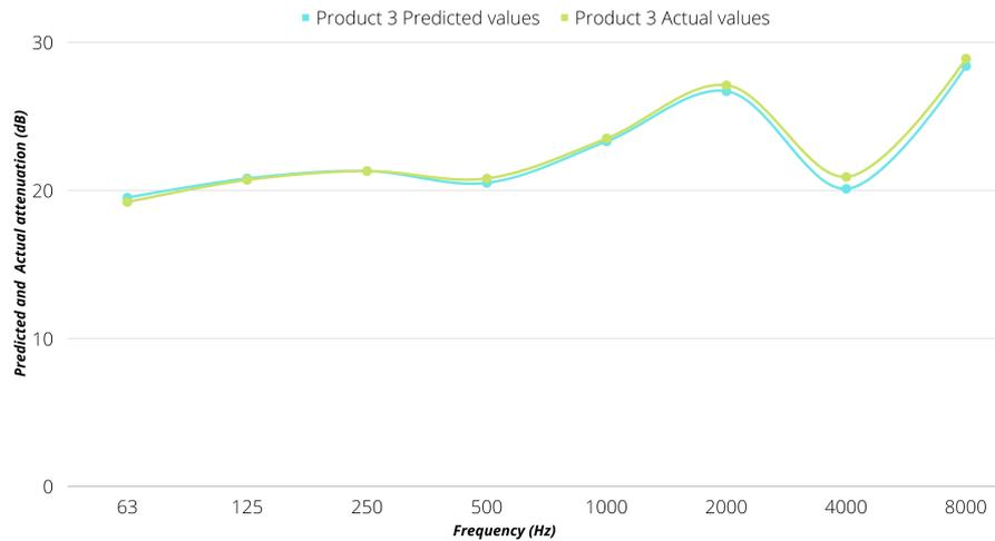
**Figure 4.7:** Actual Attenuation values (Green curve) vs Predicted Attenuation values (Blue curve) of Product 3 in mesh dataset. The x-axis is the frequency in Hz and y-axis is the predicted (Blue curve) and actual (Green curve) sound attenuation in dB. The predicted values are almost the same as the actual values.
