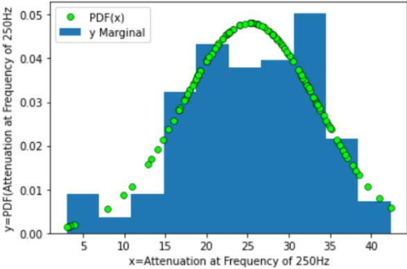
**Figure 3.26:** Histogram of attenuation at frequency=250 Hz and the green point represents the probability density function of attenuation at frequency=250 Hz. The histogram of attenuation at frequency= 250 Hz more or less resembles the Gaussian distribution. So, the marginals are assumed to be Gaussian distributed
