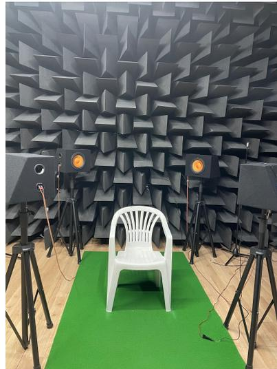
**Figure 2.1:** This picture is taken from the PZT testing laboratory and certification body in Germany. This setup shows the subjective testing method where the subject is seated at the centre of four loud speakers. The subject is given a button to press when he/ she first hears the sound that is played at a particular frequency and it is his/ her threshold of hearing. The hearing threshold is measured with and without the earplugs. This testing is carried out one by one for all 16 subjects.
