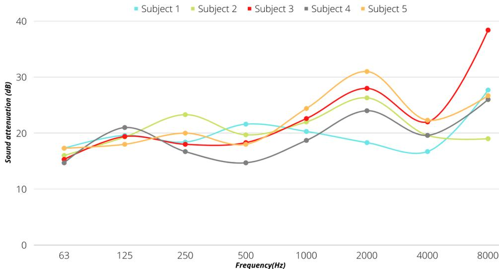
**Figure 3.25:** Frequency (Hz) vs Attenuation (dB) plot for first five subjects of Product 3 in in Mesh earplugs. The same product tested on different subjects results in different attenuation values for each frequency
