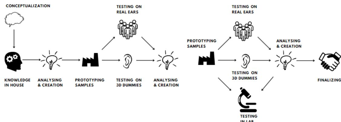
**Figure 1.1:** During the earplug designing phase, the earplugs are conceptualised, analysed and prototyped. Then these earplugs are tested on subjects and on ear simulators to assess the attenuation level to check if the earplug provides the required attenuation level. If not, these earplugs are discarded and a new earplug is redesigned until the required noise attenuation level is achieved. Hence, the earplug development and testing process is iterative and is a trial and error method [4]
