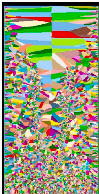
Fig. 16. Grain structure prediction in an Al-Si alloy cast ingot [230].
