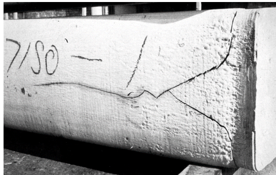
Fig. 19. Cold crack in a 7xxx DC ingot.
