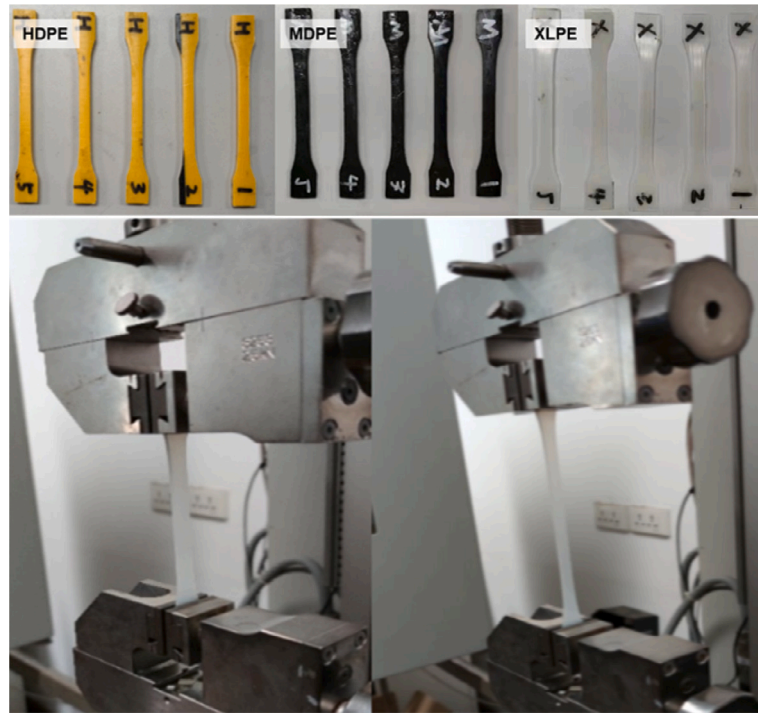
Fig. 9. Test samples of polymers (top) and photographs of material tests (base).
