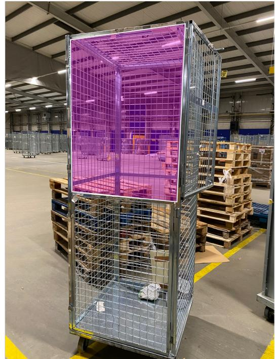
**Figure 2.12:** Photo of a roll container as found in many logistical warehouses. The only access into the container is via the opening in the top half of one of the sides of the cart. The magenta plane shows the access point to unload the ULD through.
