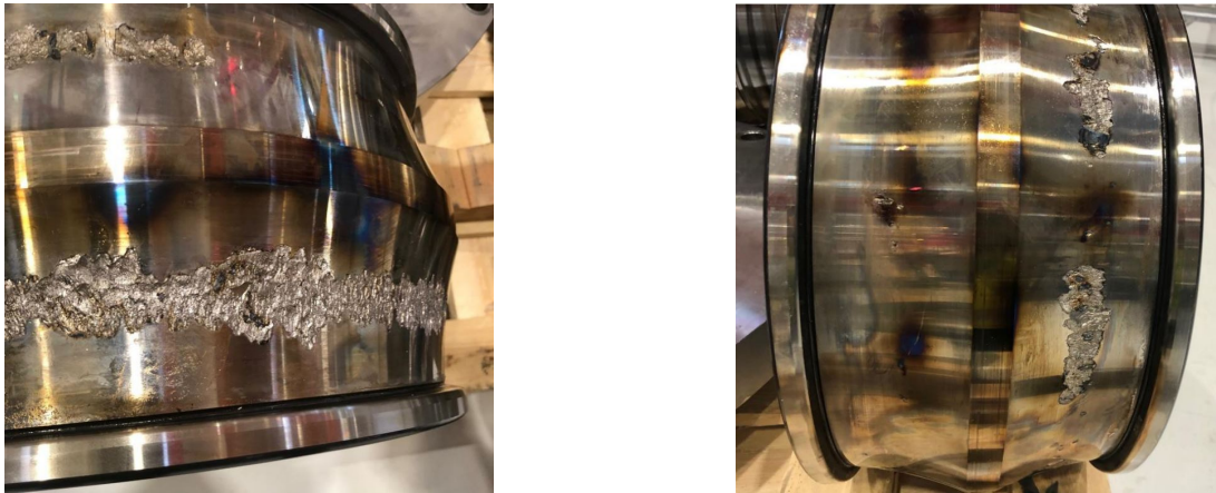
Figure 3.3: Heavy spalling on the inner raceways of a bearing in a marine vessel thruster assembly [26]
