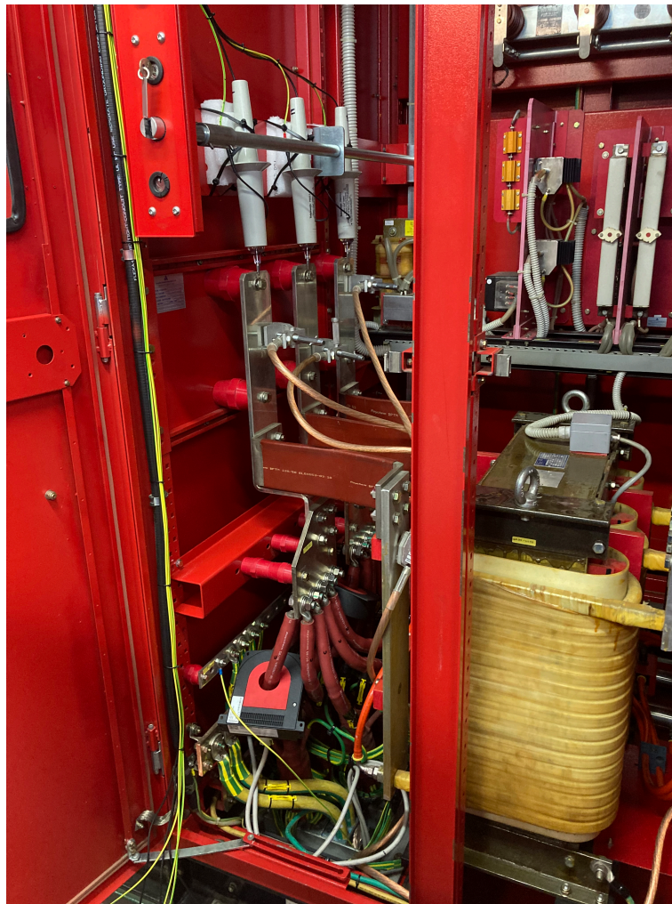
Figure C.1: Sensor setup inside the VFD. The HV probes are connected on top of the bus bars. The Current Transformers are connected around 1 of 7 phase cables.
