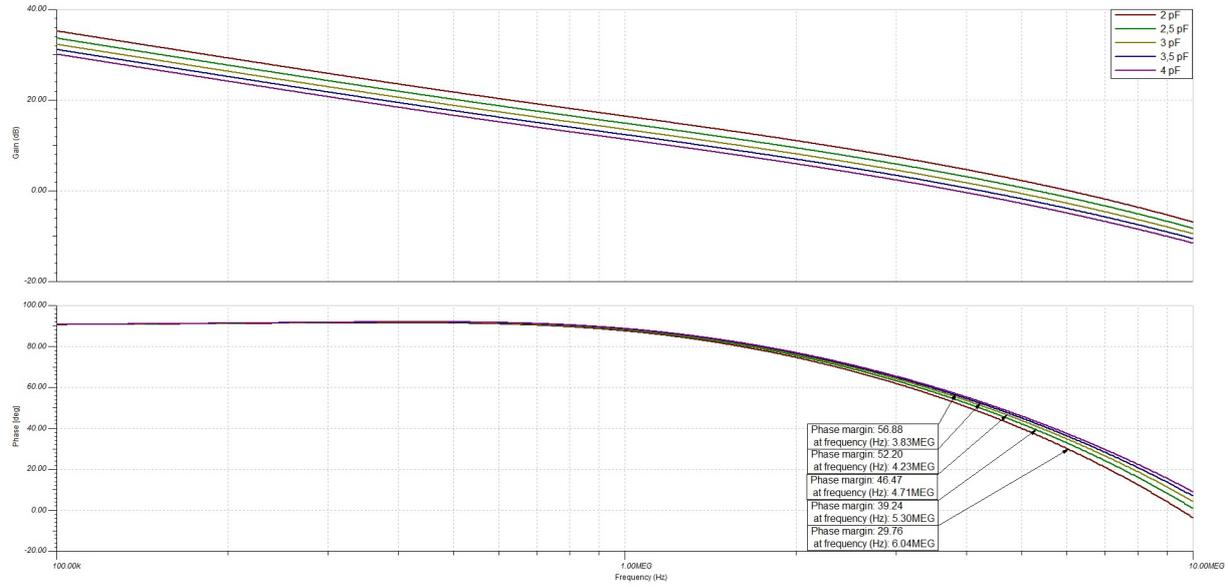
**Figure 3.10:** A simulation of the loop gain with dominant pole compensation for different values of  $C_1$ .
