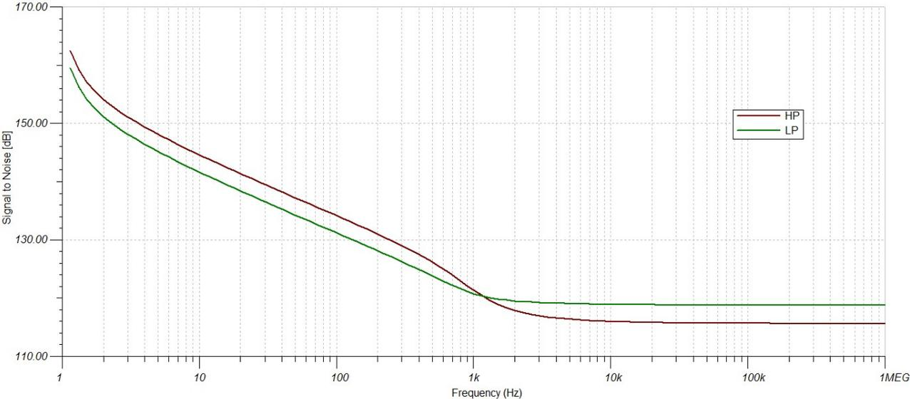
Figure 3.24: Noise-Bandwidth Performance of the Final Linkwitz-Riley cross-over Circuit
