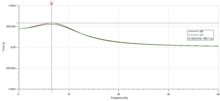
**Figure 3.20:** Delay Analysis of the Linkwitz-Riley cross-over Circuit
