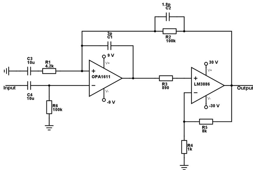
**Figure 3.12:** The fully dimensioned nested feedback amplifier
