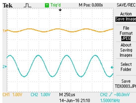
Figure 4.2: Low-pass filter at 1500 Hz
