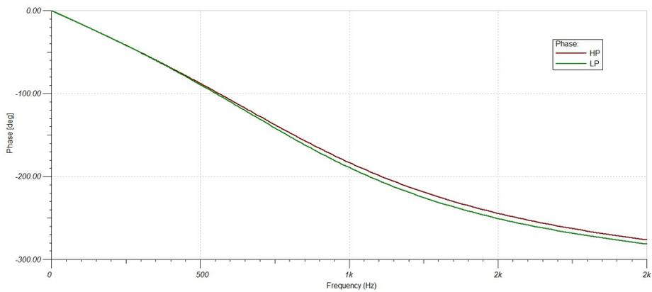
Figure 3.19: Phase Analysis of the Linkwitz-Riley cross-over Circuit
