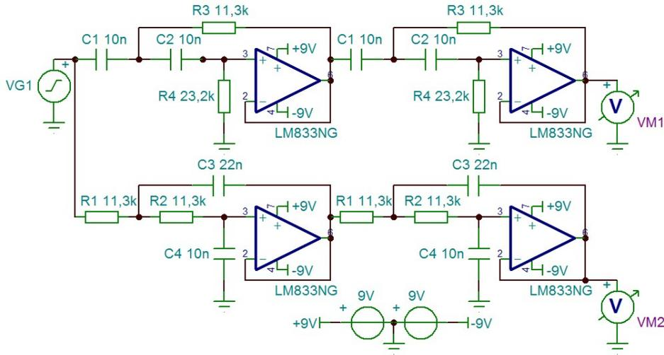
Figure 3.17: Linkwitz-Riley cross-over Circuit
