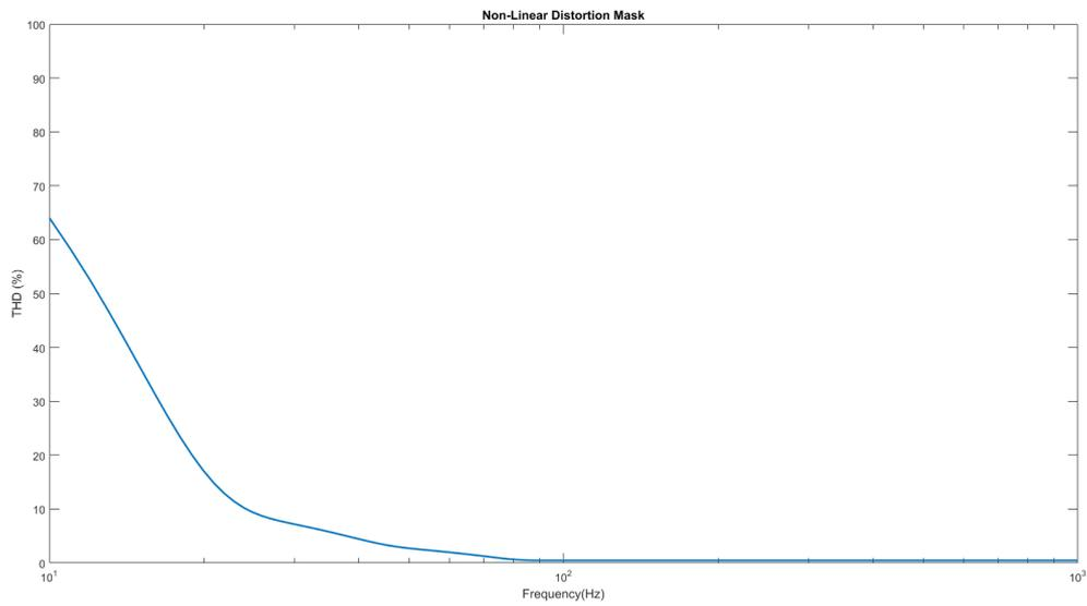
**Figure A.1:** The distortion mask created to specify the output distortion as a function of frequency.
