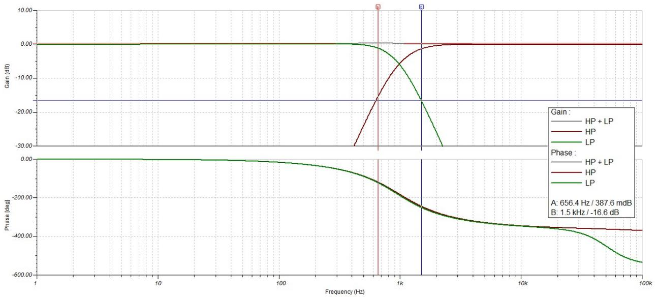
Figure 3.18: AC Analysis of the Linkwitz-Riley Cross-over Circuit
