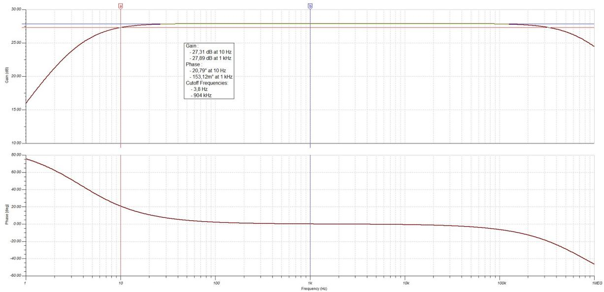
**Figure 3.11:** A simulation of the closed loop transfer after adding the DC filters to the circuit. The simulation meets specifications 2.22 and 2.23.
