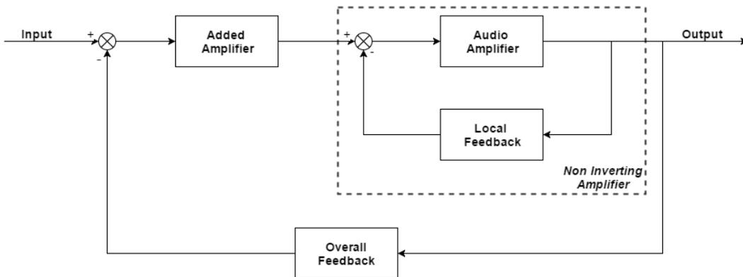
**Figure 1.4:** The control scheme of the nested feedback topology.
