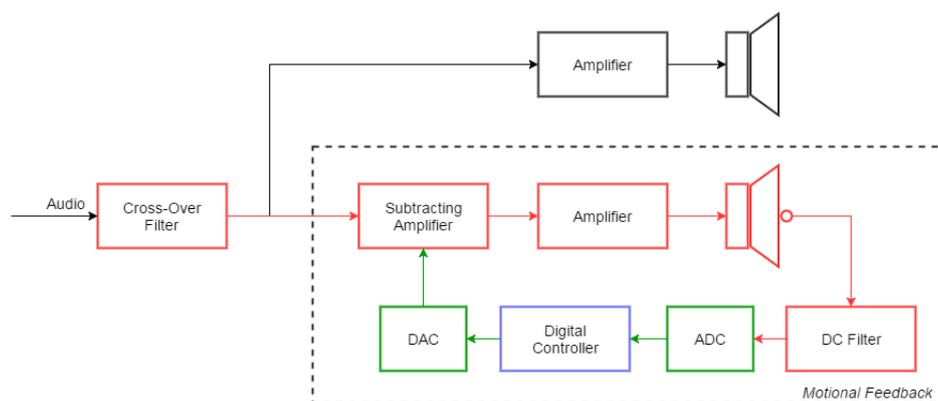
**Figure 1.2:** The motional feedback system designed by the three groups. The green parts are designed by the digital group. The parts highlighted in red are related to the amplifier/filter group. The blue part is the controller implemented by the control group. The MFB system is shown here in a two-way loudspeaker setup, where the tweeter (on top) does not use motional feedback.
