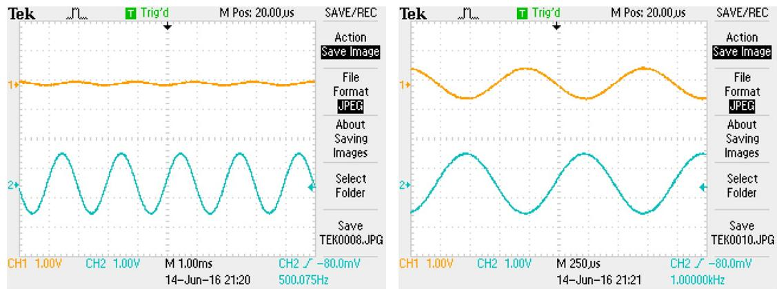
(a) High-pass filter at 500 Hz
