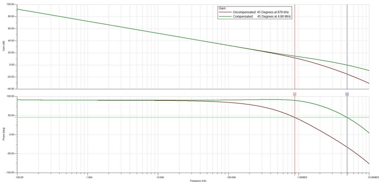
**Figure 3.8:** A simulation of the loop gain of the uncompensated and lead compensated circuits. The lead compensation improves the phase behaviour of the system.
