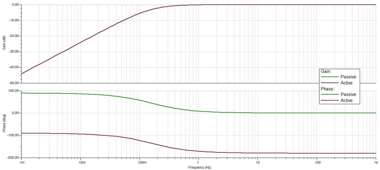
Figure 3.27: AC Analysis of the filters
