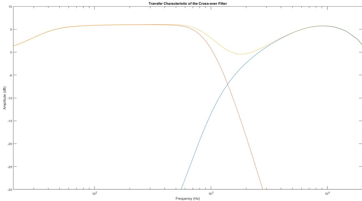
Figure 4.1: Transfer function of the Cross-over
