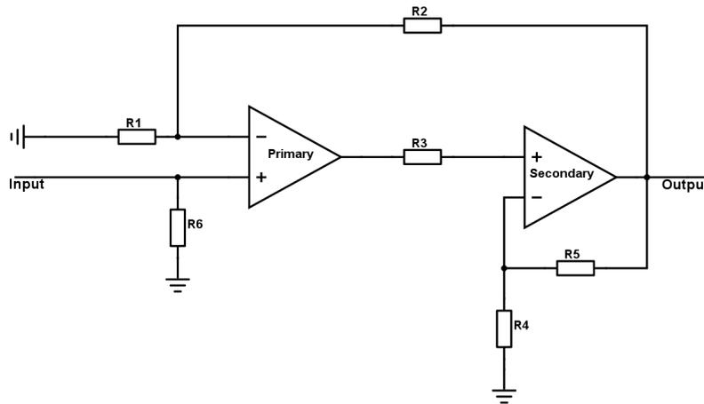
**Figure 3.5:** The topology of a nested feedback amplifier
