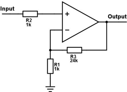
Figure 3.1: A non-inverting op amp amplifier with a gain of 28 dB as specified by specification 2.21
