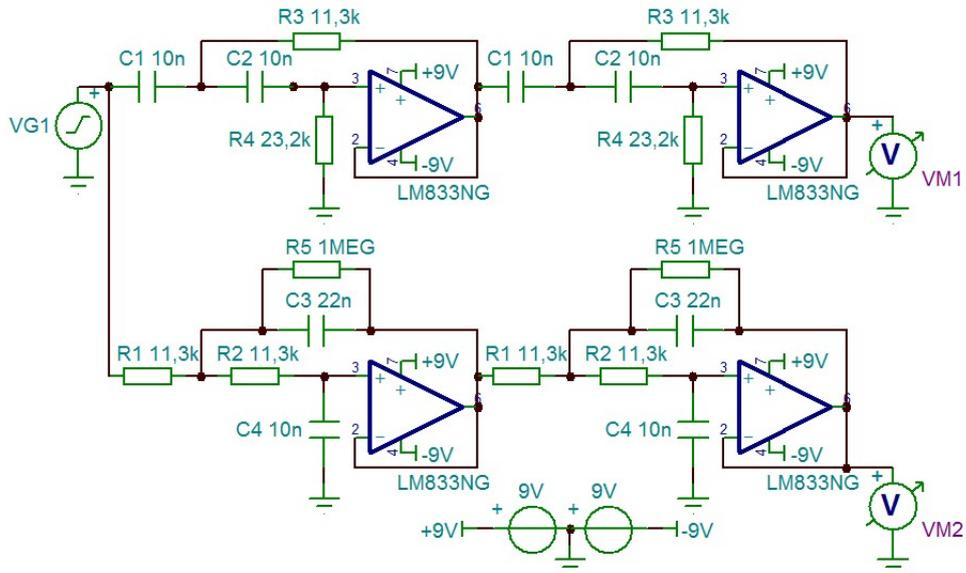
Figure 3.22: Final Linkwitz-Riley Cross-over Circuit
