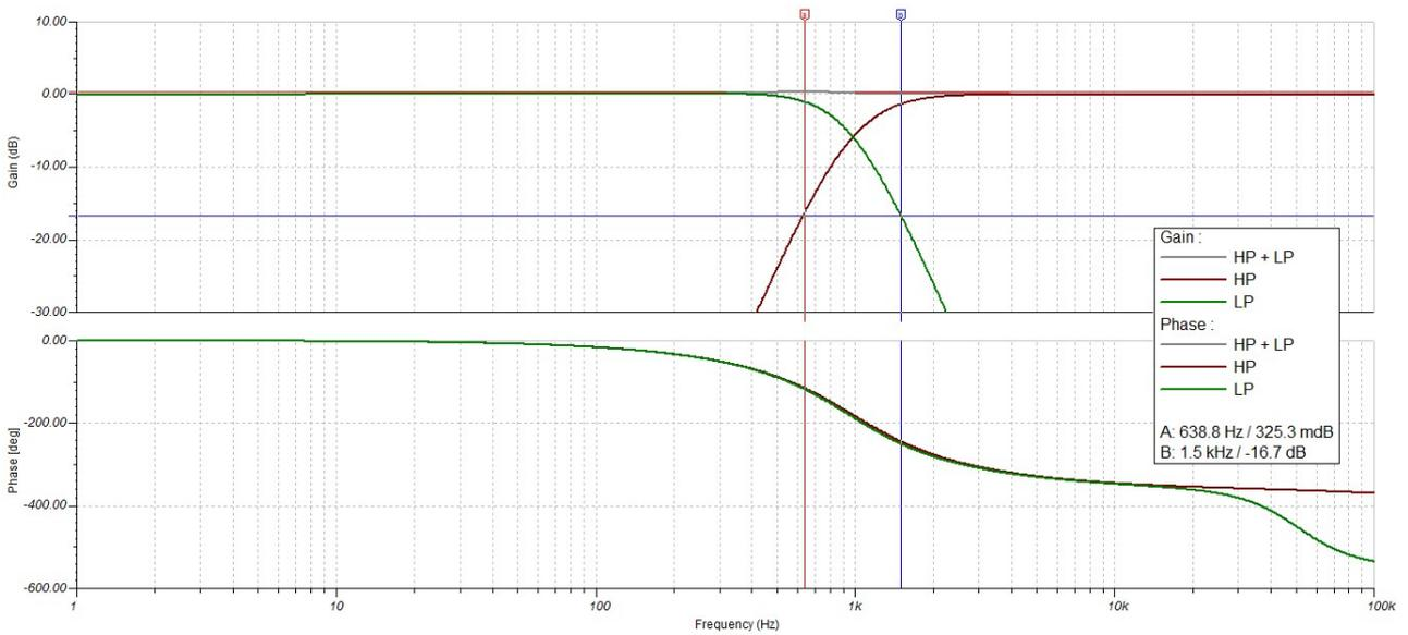
Figure 3.23: AC analysis of the Final Linkwitz-Riley cross-over Circuit
