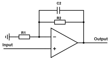
**Figure 3.7:** An amplifier where  $C_2$  is added to implement lead compensation.
