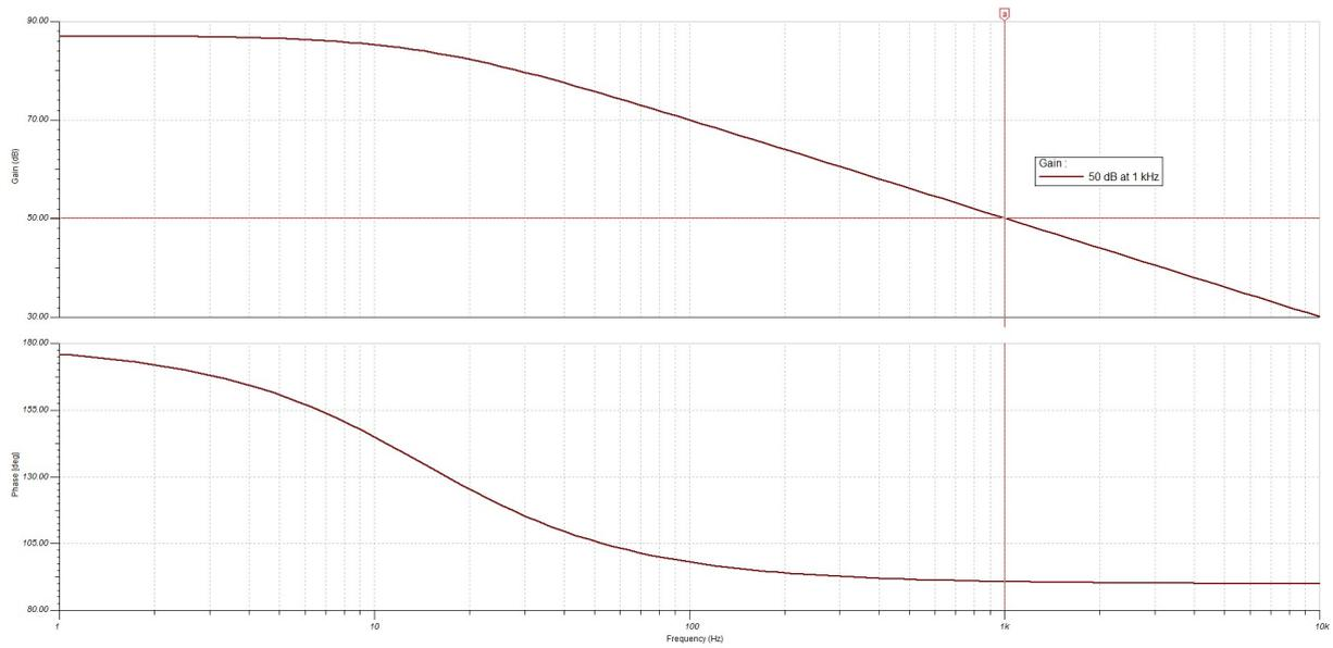
**Figure 3.3:** A simulation of the loop gain for the amplifier in the non-inverting configuration, as depicted in figure 3.1
