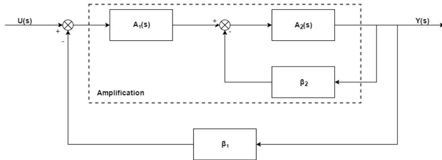
**Figure 3.4:** The proposed control scheme, where the open loop gain is increased compared to figure 3.2
