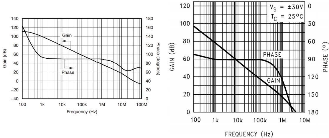
(a) The magnitude-phase characteristic of the OPA1611 (b) The magnitude-phase characteristic of the LM3886
