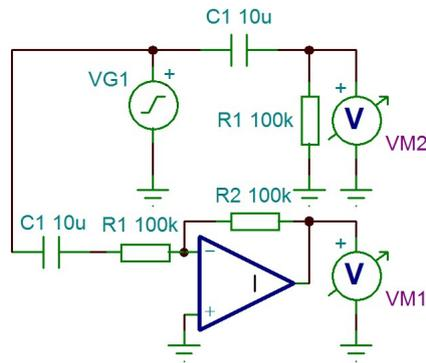
Figure 3.26: Two types of Filters
