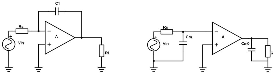
**Figure 3.9:** Two equivalent circuits. The miller effect greatly increases the capacitance at the input due to the capacitance between the input and output terminals of the amplifier.
