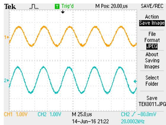
Figure C.4: High-pass filter at 20000 Hz
