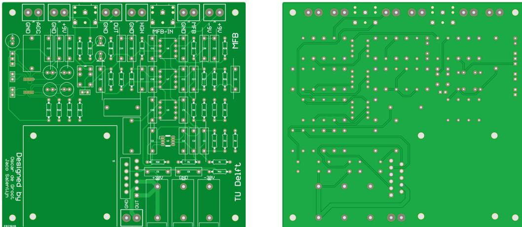
(a) PCB Design (top) of the amplifier, ADC and crossover (b) PCB Design (bottom) of the amplifier, ADC and crossover
