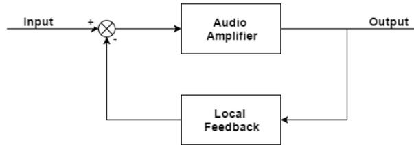
**Figure 1.3:** The general control scheme used for implementing audio amplifiers.
