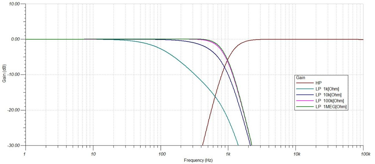
**Figure 3.21:** Effect of adding Resistor R5
