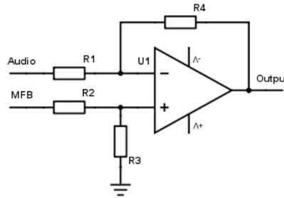
**Figure 3.25:** The topology of a subtracting amplifier.
