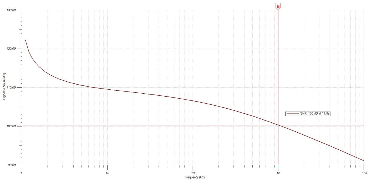
Figure 3.14: The SNR of the nested feedback amplifier.
