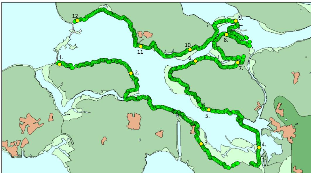
Figure A.37: Test locations (OS-1 to OS-12) to determine hydraulic loads for most dyke sections in estuary of the Eastern Scheldt (Hydra-NL).
