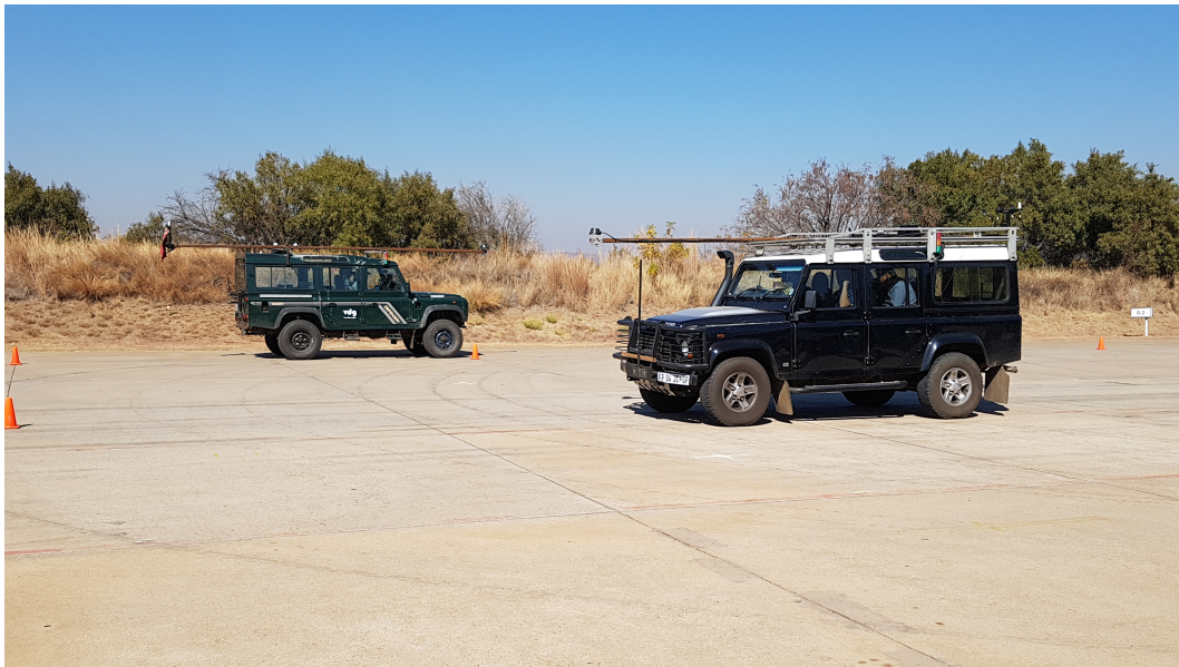
Figure 1-1: The two Land Rovers are used to test CASs for commercial entities
