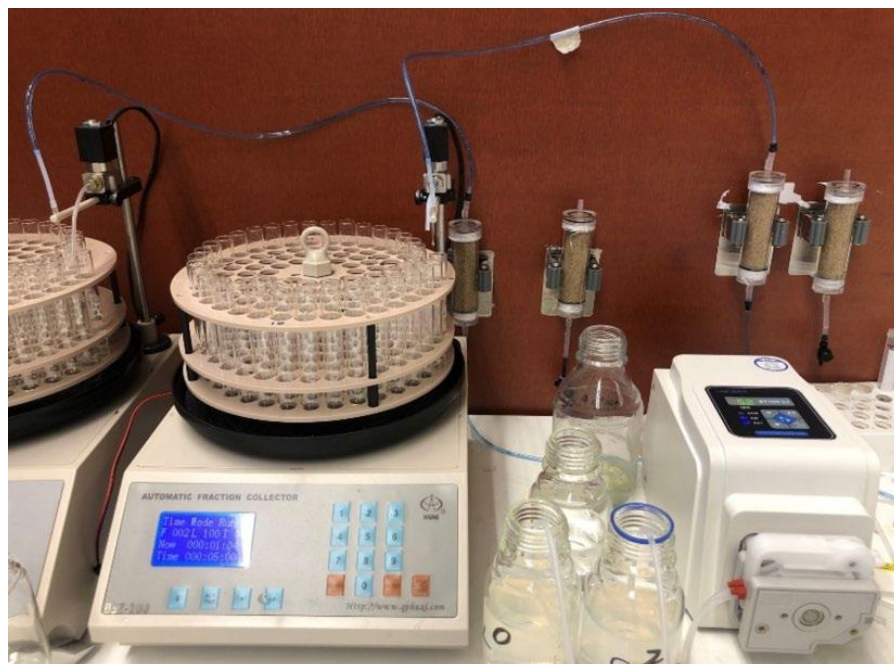
Figure S23. Photograph of the experimental setup used for NP transport experiments.
