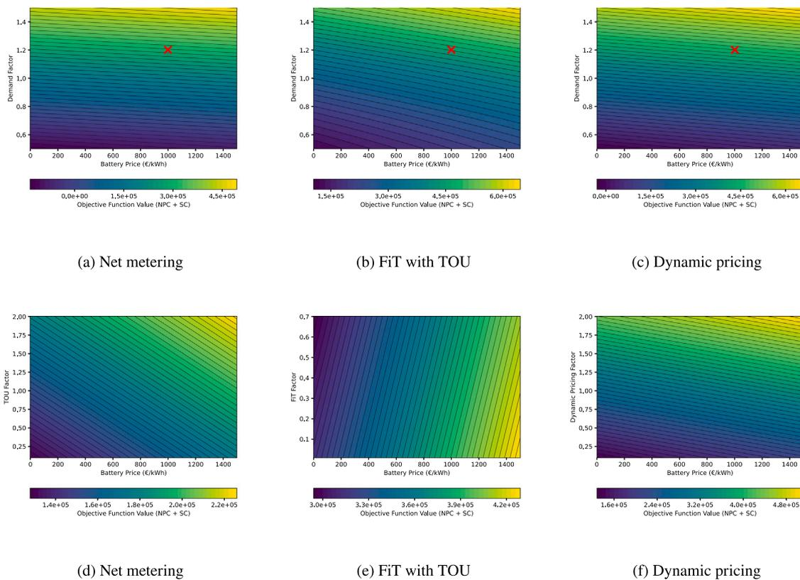
Fig. 13. Sensitivity analysis for different scenarios. (a), (b) and (c) show the effect of BES price and demand change on the objective function value. (d), (e) and (f) show the effect of BES price and electricity price changes on the objective function value.
