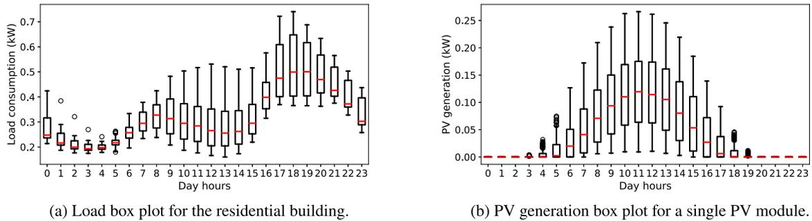
Fig. 3. Daily load and PV generation in the assumed microgrid for 2021.
