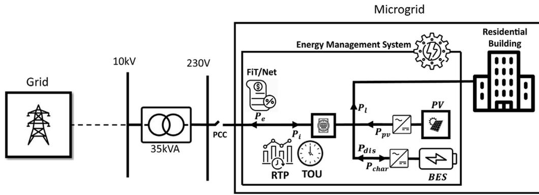
Fig. 1. Microgrid architecture incorporating a PV-BES system.
