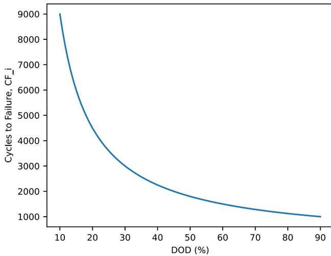
Fig. 5. Cycles to failure vs. DOD for a typical battery.
