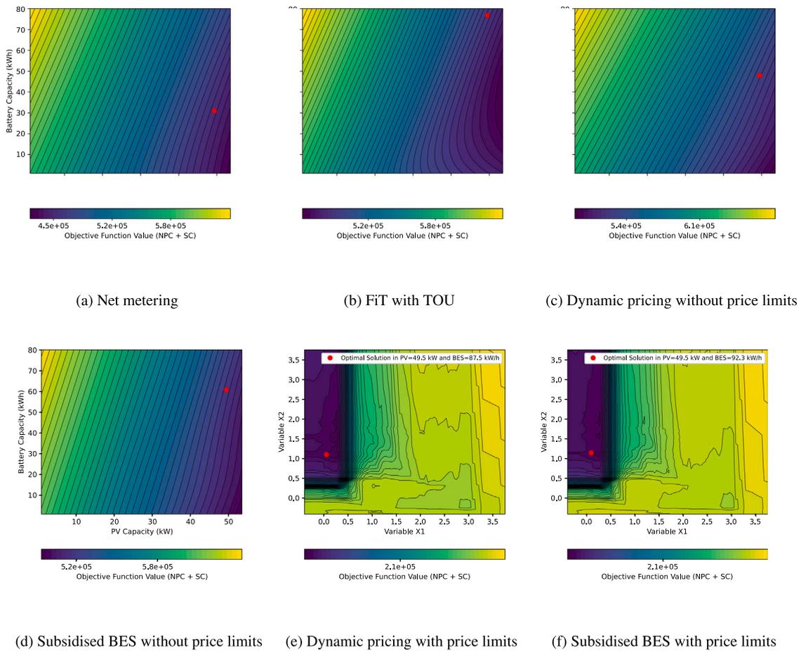
Fig. 11. Objective function values for each scenario. The red dots indicate the optimal solutions.
